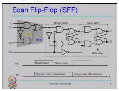
So this is the design of a scan flip-flop wherein we use a master slave D flip-flop and a multiplexer before that. So here you have the test control input, scan data input, this D input from the circuit and then this is your clock.
