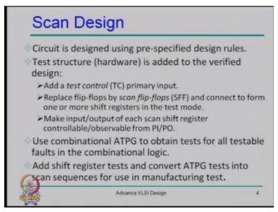
So now here I can load any arbitrary value, I can read any value from these flip-flops, but here what I need, I need at least one additional test control input that is the input that can control all these multiplexers and now here you have to replace all these flip-flops by scan
