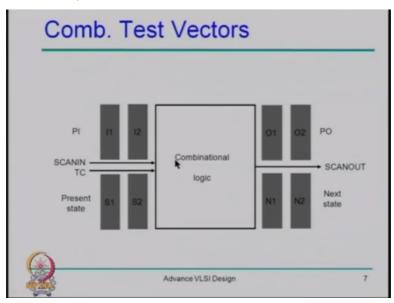
So now here how you apply test? First look at the simple combinational logic, how we apply test to a combinational logic? You have a combinational logic, you apply some input and then here you need to apply the value from the state variable. So that means your pseudo primary input and then primary input and then every cycle you are getting output then your output may be at the primary output or that may go to the pseudo primary output and you are reading that.
