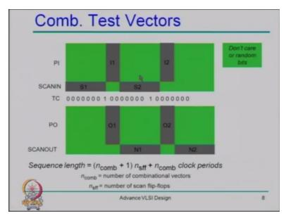
So now here in place of having this vertical S2, S1 now you need to make it horizontal so that that means here in couple of cycles you need to SCANIN the test vector in the flip-flops and then in one cycle you apply input from the primary input, capture the rest ones and then here you read the test response directly from the primary output of the circuit and then the response is stored in the flip-flops would be shifted out while you are shifting in the next vector.
