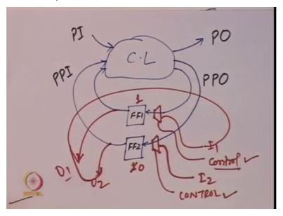
Now here if you look at a sequential circuit, if you can look at a sequential circuit, it has a combinational logic, a couple of flip-flops. So now it has some primary inputs, some primary outputs and then here the input, which is coming from the flip-flop is known as pseudo
