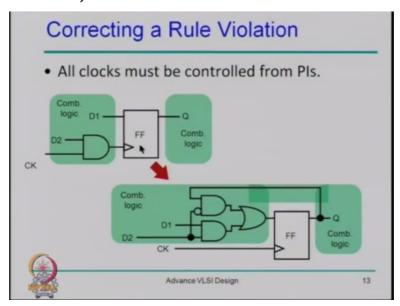
So like here for example if this is the circuit wherein you have one flip-flop and then the clock is gated and sometimes it is very easy to design this kind of gated clock circuit. So now here clock will depend on the clock and D input so that means here whenever D input is high and clock is high, it allows the value to change in this flip-flop. Now when I do not want this or we do not allow gated clock what we need to do?
