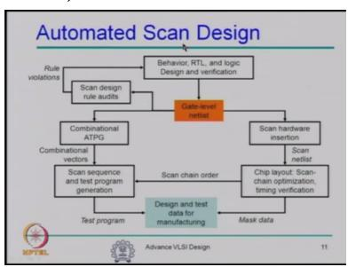
So now in general, the scan design flow is more or less automated today so when you start your design flow from RTL you synthesize your circuit to gate level netlist, once you have gate level netlist in that case here there are two things you have to do, one thing is because you have gate level netlist you have combinational logic in this, you start to generate the test vector from the combinational logic.
