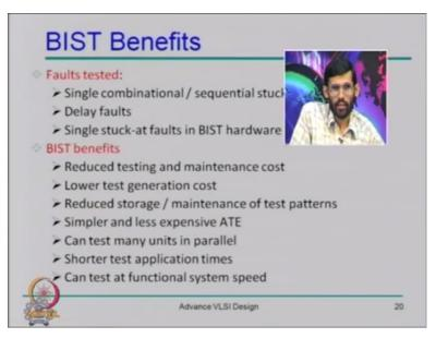
So now here if you look at what kind of faults your built-in self-test can detect? These are like here all single faults in the combinational or sequential circuit, all the delay faults, single stuck-at faults in the built-in self-test hardware or architecture. What are the benefits of this? It reduces the maintenance cost, it generate the test at lower cost, it reduces the storage or maintenance of test vectors, it is simpler and less expensive, automatic test equipment is needed.
