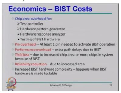
And then here in order to control all these activities here you must have a test controller that can control that means that can excide the test better and generator and analyzer at different point in time and then here you need to have some methodology to test that built-in self-test hardware. It also comes with some pin overhead so that means here at least you must have one additional pin that can say you that here now it is the time for built-in self-test.
