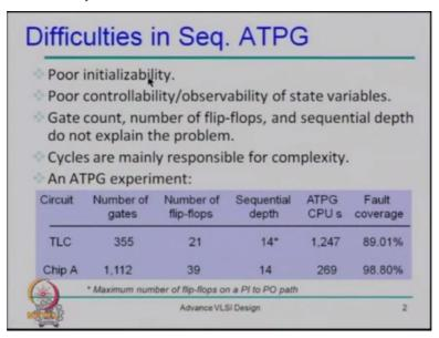
So now here look at the problems, problems are due to the poor controllability and poor observability. So that means here if we can enhance the controllability and observability of the circuit, we can make it better test evolve and hence we can reduce the test generation time and this is coming though.
