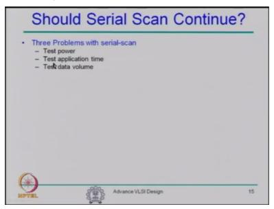
You need enormous used memory so that means the storage of the test data is also a problem. So that is additional problem that we have. The very important problem nowadays is the test power, which was not there earlier. Though here the test data volume was also not very big problem initially because at the time the circuit complexity was not that much or the circuit was too small.
