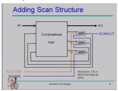
So now here as I said that we need three additional signals, one is the SCANIN, one is the SCANOUT and another is that the test control or test clock whatever we say. So now here this signal controls all the multiplexers associated with these flip-flops and then the SCANIN and SCANOUT, provide you the shift path. So now you can load any value and when you generate the test you need to generate test for the combinational logic.
