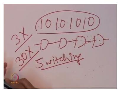
Now here what is the source of test power? So say easily you may generate a test vector wherein you may need to load a test data like here 101010 sequence because this sequence you are generating from the combinational logic. Now when you load this sequence in flip-flops what will happen because there are different adjacent bits, so in every cycle when these bits will shift every flip-flop will toggle.
