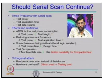
Then in order to reduce the test time or test data size here you can do the compression at the primary input and at the primary output. Compaction or compression is the widely used technique, but here again it has limited capability so these are some of the effort, which were proposed by people to take care of the additional problems, which are coming from the serial scan design.
