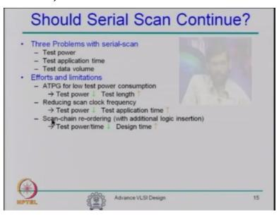
So like here some of the efforts, which are being made like one of the effort is while you are generating the test you can generate test because as we discussed earlier that one fault may have multiple tests. So you can select a test, which can dissipate less power and when you are generating test, it generates large number of access so that means here the propagation of fault effect is not impacted by those primary inputs or pseudo primary inputs.
