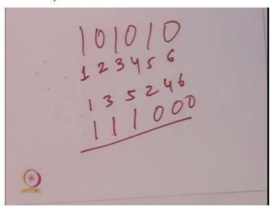
The other way is like here you can reorder these scan chain and reordering mean here say if you want to SCANIN the pattern 101010 and so now here you have 1 in flip-flop 1, 0 in flip-flop 2, 1 in flip-flop 3, 0 in flip-flop 4, 1 in 5, 0 in 6. If I can stich this scan chain in different way like here 135246 in that case here how I need to SCANIN, I need to SCANIN 111000 and hence I can reduce the number of transitions because now in every cycle there would be only one transition here.
