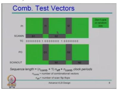
So now here if you look in this expression in that case here, this is n combinational logic so that means the number of test vectors + 1 into number of flip-flops + number of test vectors. These many cycles it will take, so it will elongate the test time. The elongation of test time directly results into increase in the test cost, but it greatly reduces the test generation effort.
