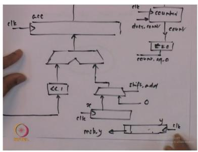
So here is a big accumulator. This is a clock resistor; I call it accumulator. This accumulator is going to be taking at times just a shifted version of itself or the result of the ALU addition, okay? So when you test the shifted version of itself it is like will regard it as if it is the adder is adding 0 to it, okay. So in the case of shift and add will be passing this accumulators content through 1-bit shifter and putting it at this adder,
