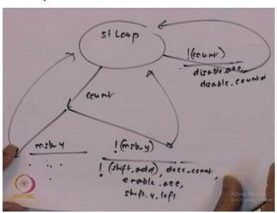
Or as the matter of test you might prefer a variation of this instead of this might feel that this could suffice as it is if count is not 0 it will depend on MSB Y and lot of this signals are specified here if MSB 0 then just shift do not add decrement counter, enable accumulator and so on so forth what else shift Y left and similarly here, we go to this, we go to this. If count where 0 then we might prefer to use a single state machine,
