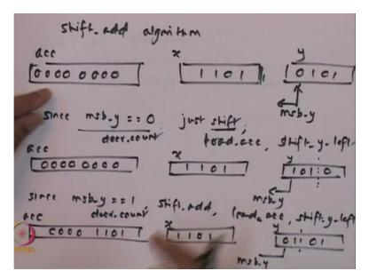
The shift the so call shift add approach, shift and add algorithm which is very easy to hardware and that is what we are going to see it as FSM + datapath is as follows. So, we are going to maintain an accumulator where the multiplication will accumulate that accumulator will be initialized to it will be sufficiently big accumulator capable of storing the product, this is X and this is Y.
