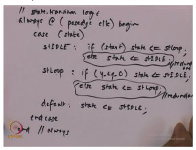
So the Verilog for generation of this I mean like the state machine. So, first let me describe the state transition logic. State transition is taking place at the triggering edges of the clock that is a passage of positive edge at the clock, okay? So, typically it is going to be described using a case statement depending on what the current state is we had different cases. The current state is state idle then we stay in the same state as long as start is 0.
