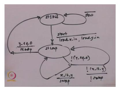
So now we have started working, I mean on the protocol like where this start signal is quickly responded to and that required a use of state called state idle which the system is kind of waiting for the start signal to the asserted and when start is not asserted staying this state. Once the start signal is asserted then the system in the next clock cycle would move to a state St Loop, okay.
