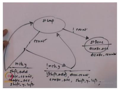
So, quickly like from this state we check whether count is 0 or not, if count has dropped down to 0 we know that this computation is finished, okay? Let see what to do whether to go back in this state or not. This is important this is when the computation continues. If count is not 0 then it would depend on whether MSB of Y is non 0 or whether MSB of Y is 0, okay? If MSB of Y is non 0 then we know that, not only we had shift but also add X.
