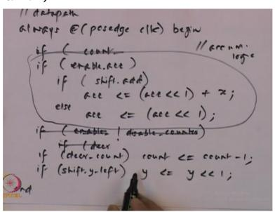
So let us describe the datapath in Verilog. So, this will also consider it understanding of how Verilog semantics capture the datapath as well as the controller. So the datapath, datapath is synchronous system, right? So what is happening if let us make is of single cycle controller if
