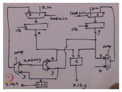
So the datapath for GCD just to consolidate the picture in your mind. I will repeat quickly draw bit more neatly. This is the X resistor which is driven by output of a multiplexer and this multiplexer is controlled by output of a controller with a signal load Xin and when this load
