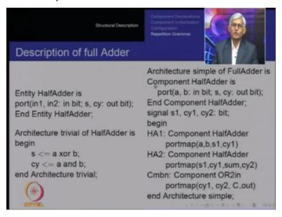
We are declaring s1, carry1, carry2 as the internal signals; s2 will be directly mapped to the port sum and then we place these components. There are two instances of the half adder so HA1 component half adder, remember we have declared the component half adder here and portmap these ports that had been declared here to a, b, s1 and carry1 that is this half adder, this half adder inputs are mapped to a and b and the outputs are mapped to s1 and carry1.
