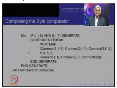
And this is the interesting part, this is the middle part and if I is greater than 0 and I less than 7, then no port signals are involved and then we say generate and then we say that the component to be used is the bit part and the port mapping is the array at the input and the array at the output, only aI and bI are the bit specific signals which will come. So by using a generate then we have used all the component parts.
