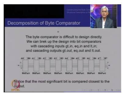
We have not instantiated generics and that can be shown by having a byte comparator, which compares two bytes and each internal components is a bit comparator. So essentially we are making a byte comparator to give you an example of a hardware, which uses repetitive hardware components and assume that you have input bit comparators and these bit comparators will then be stacked eight of them.
