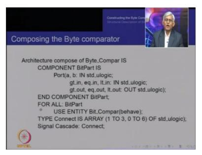
So now you have this architecture compose of byte compar IS and then we declare a component bit part with these ports and these outputs greater than in, equal in and less than in as the inputs because you are concatenating design and greater than out, equal out and less than out as outputs. So each bit comparator has a and b as inputs, but it also has concatenating inputs from the previous comparator and it produces three outputs which is greater than equal or less than as outputs.
