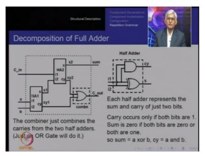
Notice these are the internal signals of the FullAdder, s1, cy1 and cy2 are the internal signals remember s2 is directly mapped to a port and therefore need not be declared as an internal signal. Similarly a and b are directly available as ports. So it is a carry in, so these do not have to be declared as internal signal. So at the result it is only s1, s2, carry1 and carry2, which are internal to this architecture and that is what we are doing.
