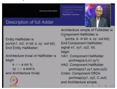
Now this is how in VHDL will describe the FullAdder. Entity half adder is; this is what we need for the FullAdder. Port in1, in2 as inputs of type bit and port s and carry these are outputs of type bit and this ends the entity half adder. The architecture trivial of half adder is and you assign to s a xor b and assign to carry a and b and this is the trivial architecture. Now architecture simple of FullAdder is now we declare a component type half adder.
