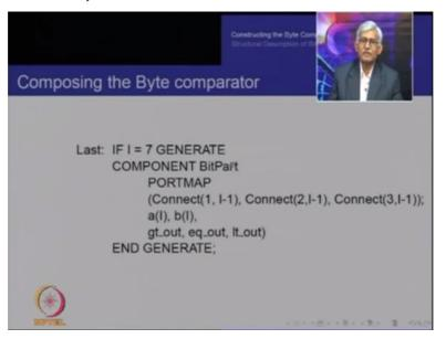
Also the last part is unique if I equal to 7 then generate and it is very similar except that the inputs are now cascaded, but the outputs are the port outputs.
