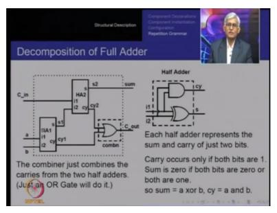
So let say that we cannot design a FullAdder from scratch. We would like to describe it in terms of a simpler circuit called a half adder, which adds only two bits at a time. So then we can decompose the FullAdder into two half adders. The first half adder adds a and b and produces two outputs sum1 and carry1. This sum1 is then combined using a half adder with the carry in.
