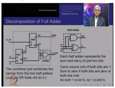
Recall this is HA1, the inputs are mapped to a and b. the outputs are s and s1 and cy1 and then s1 and carry in are the inputs to half adder 2 and sum and carry of this are mapped to sum directly here, which is the port signal and cy2 is then mapped to the input of this R gate.
