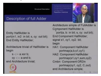
So that is what we are saying HA1 is component half adder, portmap to a, b as input, outputs are s1 and carry1. HA2 is also the same component half adder and it is port mapped, two inputs are s1 and carry1 now and outputs are the sum of the entity and carry2. Now we need to combine the two carry into a single carry and that instance is called combination. We have a previously declared component OR2.
