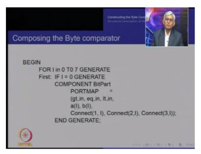
And this is the example that we wanted to show then we will say for I in 0 to 7 this is going for all the bits generate and then we have a special case if I equal to 0 generate component bit part and when we map it in case of I equal to 0 we map it to the port entries, the 0 part maps directly through the entries of the entity and the outputs are aI, bI. These are the other two bit inputs.
