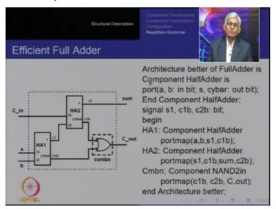
So now you have HA1 with a better architecture, HA2 with a better architecture both giving carry bars and the combiner now is the OR of negative inputs, which is in other words a NAND. So now we have the architecture better or FullAdder, which uses component half adder so we declare a component half adder with these ports with signal s1, c1b, c2b and we instantiate HA1 and HA2, which is component half adder portmap and so on.
