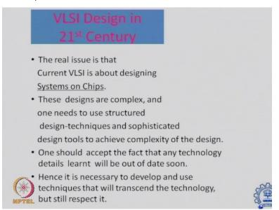
So what is VLSI design? In 21st century the real issue is the current VLSI's about designing system on chips, okay. Now these designs are extremely complex and one needs to use structured
