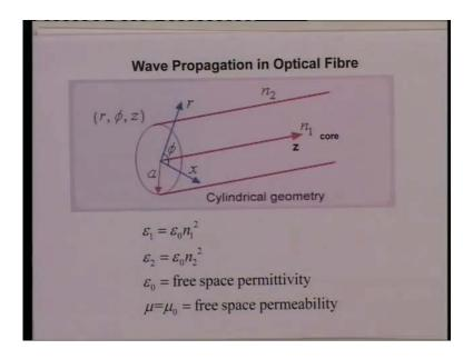
So, for wave model essentially we define first appropriate coordinate system for the optical fiber, which is cylindrical coordinate system. So, we assume that the core of the optical fiber is a solid glass rod having refractive index n 1 and then we assume that the cladding is of infinite size with a refractive index n 2.
