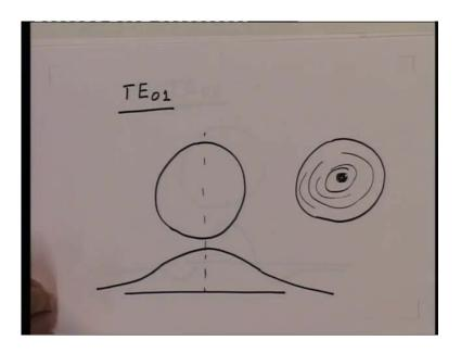
So, if I say that I have a T E 0 1 mode and then this mode is circularly symmetric and does not say 0 crossing an radial direction. So, if I take this and try to draw the fields for this, it is a circularly symmetric. So, if I draw the field distribution this the function of radial direction, the field distribution would go something like this .No 0 crossing is reach till the end and them the field is decays exponentially in the cladding.
