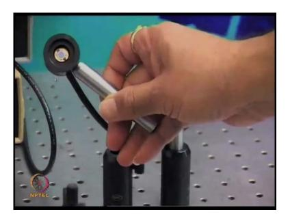
And this is the optical detector; you see this is the inner region here that is the actual optical detection device. When light falls on this, you get a photocurrent and the photocurrent is collected, and passes through this cable which is then amplified.
