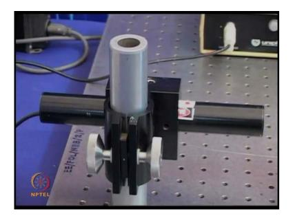
This is what is called the optical bench on which different optical components can be mounted. And this is a source, which is a helium neon laser. This is a power, which is supplied to this laser from here. And this is a tubeless structure; the laser light comes out from this end.
