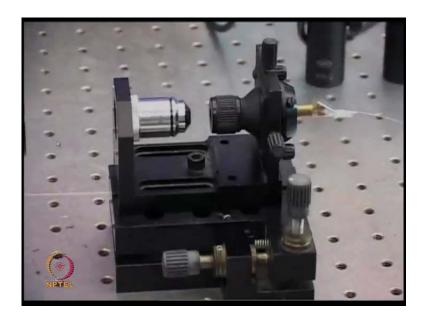
We use Helium Neon laser, because it gives you red color light and for laboratory experiments, this is in the visible range. This is assembly, which is used for aligning the optical fiber with a laser beam.
