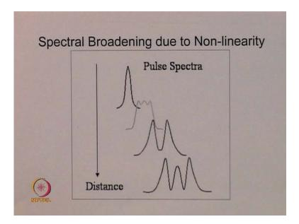
So, if I look at the self phase modulation, the phenomenon essentially looks like this. So, in the self phase modulation, because of nonlinearity we have the phenomena, what is called, spectral broadening. The time function is not changing, the pulse in time domain remains exactly intact, only thing it gets frequency modulated and because of that frequency modulation, you get the widening of the frequency spectrum.
