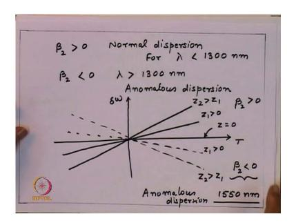
So, we have seen, in case of the dispersion the frequency chirp could be either positive for the normal dispersion or it could be negative for the anomalous dispersion regime. That mean, if you are working at 1550, then the dispersion is anomalous and then the chirp frequency chirp is negative.
