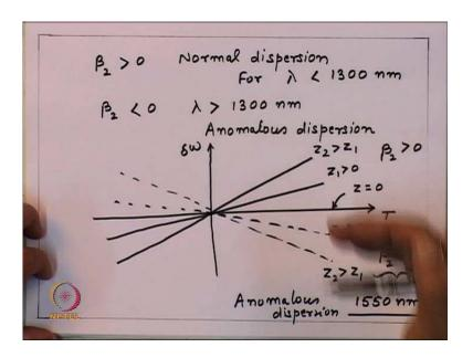
So, inside the optical fiber we see, beta 2 greater than 0, this we call as the normal dispersion and this happens if you look at the refractive index for optical fiber, this happens for wave length less than 1300 nanometer.
