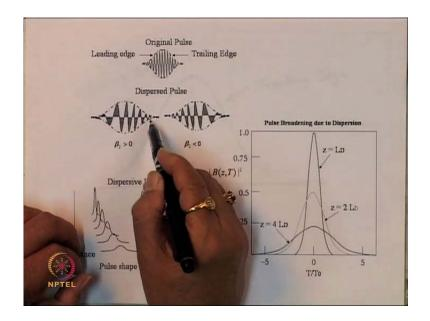
So, you see now that depending upon the situation, we may have situation like this you have the original pulse, which is like this as inside, the which is given as carrier. And you see there is a same frequency everywhere, when the pulse starts moving on the optical fiber and there is a dispersion.
