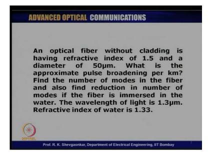
In this lecture, we are going to solve some problems related to optical fibers. Let us look at this first problem here. An optical fiber without cladding is having refractive index of 1.5, and a diameter of 50 micrometer. What is the approximate pulse broadening per kilometer on this fiber? Find the modes in the fiber and also find reduction in number of modes, if the fiber is immersed in water. The wavelength of light is given as 1.3 micrometer, and the refractive index of water is 1.33.
