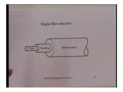
So we have solid glass rod here which is score and you have a cell which is surrounding it which is called cladding. The size of this total thing core and cladding together is of the order of about 125 microns.
