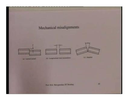
So, either the fiber could be laterally misaligned that mean the two tips of the fiber may not be axis may not align the x-ray will be slightly displaced, one possibility. Other possibility is that there may remain small air gap between the two tips of the fiber and this is more common in that temporary joint which we got with the tubular pipe the rubber pipe. Third possibility is that there will be a small angular misalignment between the 2 fibers.
