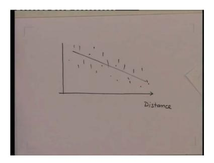
So, in fact if we just transmit one pulse and if you take the signal and plot it as a function of distance, the signal will not have a trace like this, but, signal actually will look something like that. Something like this because the signal is completely submerged into the noise.
