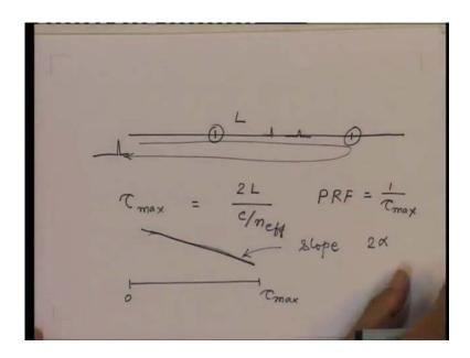
Firstly, you will note that for every pulse which is launched, that returns signal or eco will be spreaded over a time which is this time, which is tau max; that means, if we had another pulse transmitted within this time, we will not know whether the received signal is because of the previous pulse or the next pulse. In other words there has to be a minimum separation between the two pulses which should be tau max which essentially is given by this.
