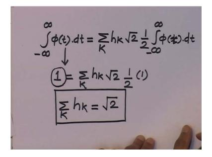
So, we will put this, in this formula, and so what we will get is. And now integration of phi of t; phi of t is in a way responsible for giving us the low pass filter, and psi of t gives us the high pass filter. So, as for as psi of t concerned, when we integrates psi of t, the integration goes to 0, but that is not true in case of phi of t. So, this integration of phi of t,
