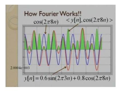
And when we take the dot product between the basis function and the underlying signal, then that gives us more positive part than a negative part, which is shown in green in this particular slide. And when we do the integration of this green part, area under this green curve, then that gives us a peak corresponding to that particular frequency. And that is how we will end up with two peaks, corresponding to two frequencies, present in this particular signal.
