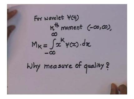
We have already noted few points, and that is for a wavelet; say psi of t. The k eth moment, can be written as, of course over the interval minus infinity to plus infinity, can be written as M of k, integration from minus infinity to plus infinity x of k psi of x d x. And then we pose this question, that why this is a measure of quality, and honestly speaking, to answer this particular question, we will go back to, what we have been doing in the Fourier domain.
