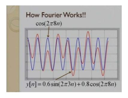
And when we stimulated this signal with the basis function, which is cos of 8, then we realized that there is huge amount of correlation. The correlation index is very high, and that is because this particular frequency is actually present in the original signal.
