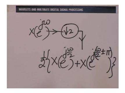
So, in down sampling if we have X e raise the power j omega here, what we get here is half X e raise the power j omega by 2 plus X e raise the power j omega by 2 plus minus pi. So, essentially, an alias is created.
