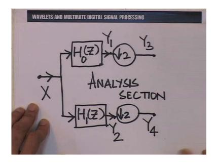
So, with that background let us recall the main structure or the prototype structure of a two band filter bank once again. Recall, that we have an analysis section and a synthesis section. We shall denote the analysis section filters by H 0(Z) and H 1(Z), these are followed by down samplers; this is the analysis section.
