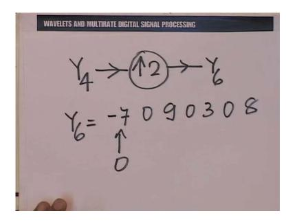
So, Y 6 would appear like this, minus 7 and then a 0, 9 and then a 0, 3 and then a 0 and finally, 8; as expected again of length 7. Now, I need to subject these to the action of the synthesis low pass and high pass filters. So, of course, we have the upper one, that is Y 5, which we have here being subjected to the action of the synthesis low pass filter and Y 6 here being subjected to the action of the synthesis high pass filter. So, let us do these two operations.
