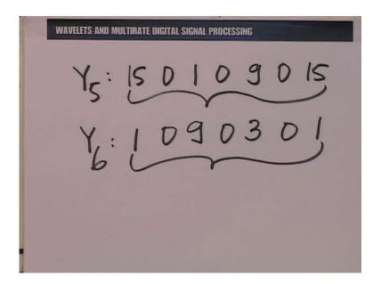
So, Y 5, it is essentially Y 3 up sample by a factor of 2. So, I put back Y 3 for your sight and Y 4 for your sight. So, when I up sample Y 3 by 2, I would get 15 0 1 0 9 0 and then 15, and I am back to a period of 6. So, as expected, when I up sample I would have a
