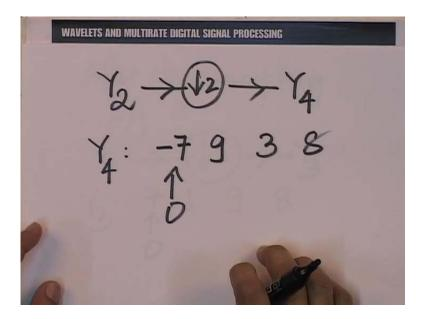
So, when we down sample Y 2 by 2, we get Y 4 and Y 4 looks like this at Y 4. Now, let me put down Y 2 once again to show you. So, when we down sample this point comes to 0, this point would come to 1, this point to 2 and this point to 3. So, we have minus 7 at 0, 9 at 1, 3 at 2 and 8 at 3 and as expected, the result after down sampling here is of length 4 and the result after down sampling here, the second one with Y 4 is of length 4 2. So, that is quite clear and as expected.
