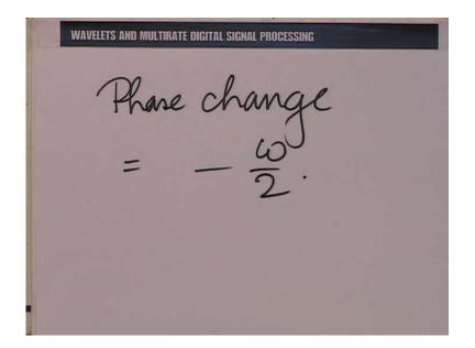
So, phase change in the analysis low pass filter is essentially minus omega by 2. I would similarly expect that you work out the phase change for the high pass side of the analysis filter bank and the magnitude change. We have done that before. So, remember, when we take a sinusoid as the input we keep getting sinusoids after filtering. But what happens after down sampling?
