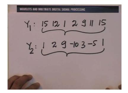
So, the output at Y 1 is, of course, obtained in this region. So, as I said, please do not forget this is of infinite length sequence, but I am only focusing between 7 and 7 here on the output. So, I would get Y 1, essentially, 7 plus 8, that is 15; 5 plus 7, that is 12; minus 4 plus 5 and that is 1; 6 minus 4, which is 2; 3 plus 6, which is 9; 8 plus 3, which is 11 and 7 plus 8, which is 15 back again.
