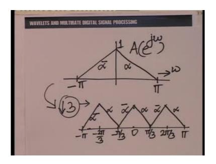
So, essentially there is a compression of the frequency access by a factor of 3; just to take an example, suppose we have the spectrum that looks like this, so this is a typical prototype spectrum as you recall; if you have the spectrum which looks like this, of course we list the same, this would be periodically repeated at every multiple of 2 pi; on up sampling by a factor of 3, we would have a spectrum that looks like this.
