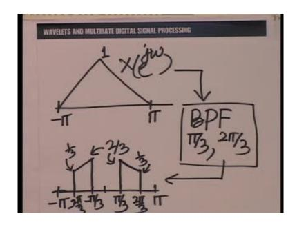
So, if we take the prototype spectrum X e raise the power j omega, subjected to the action of the band pass filter between pi by 3 and 2 pi by 3, we would get (()), only between pi by 3 and 2 pi by 3; this would be 2 by 3 here and 1 by 3 there.
