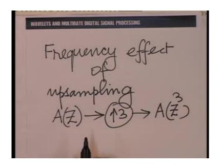
But before that, we need to see the effect of down sampling and up sampling on the frequency response. So, up sampling is easy to deal with; let us recall what happens when we up sample. So, you will recall that, if you have let us say an A Z, we infet into an up sampler by a factor of 3, what emerges is A Z cubed.
