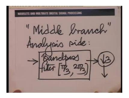
On the analysis side, the middle branch is essentially a band pass filter between pi by 3 and 2 pi by 3 - an ideal band pass filter of course - followed by down sampler of three. And let us take again the prototype spectrum, and see what happens, when we subjected to this analysis middle branch.
