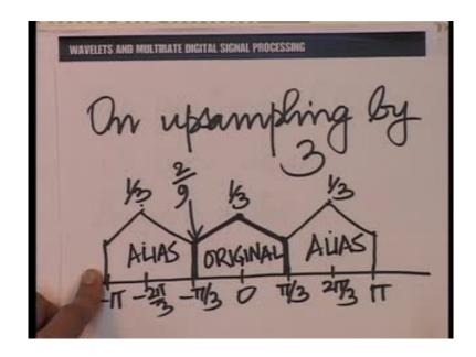
So, shape is all the same, except that, this is the 1 by 3 at the top and 2 by 9 there. Now, once we sit so clearly on this diagram, it is very easy to understand, what happens when we subjected the action of the synthesis filter. The synthesis filter is again an ideal low pass filter, cut off pi by 3, and once again we recognize if we well that, this was really the so called original spectrum and these were the carbon copies of the aliases.
