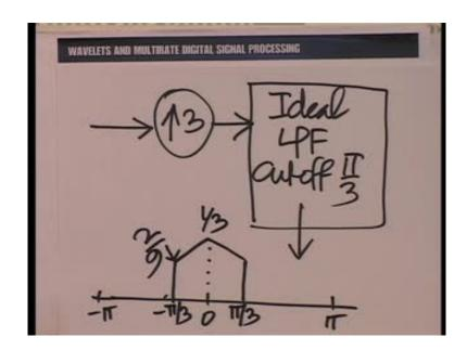
So, what the synthesis filter does is, essentially to retain the original and destroy the aliases; and therefore, what we have left after the synthesis filter. So, once we subject this to up sampling by 3, and then the synthesis filter, the ideal low pass filter with the cut off pi by 3, what we get here is essentially the original spectrum, but multiplied by a factor of 1 by 3, that is all, that is the only change.
