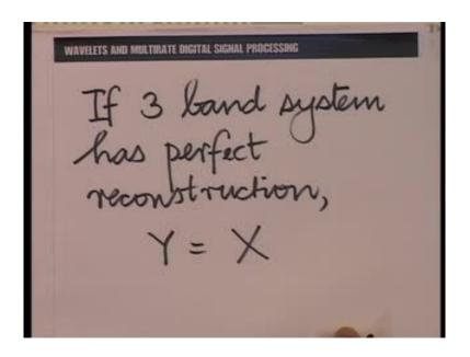
If the 3 band system is a perfect reconstruction system, Y is equal to X. When we do admit a few modifications of X and we should just recall them for a couple of minutes, we do not mind if X is scale by a constant, we do not mind if X is delayed by a constant delay; of course, what we mean is an integer delay, which operates uniformly at all times.
