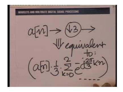
So, effectively what we have done, is to multiply the original sequence by this periodic sequence; subsequently, we reduce the Z cube to Z. So, what we are saying effectives? You have taken, if we down sample a of n by 3, it is equivalent to multiply a n by 1 third summation k going from 0 to 2 e raise the power minus j 2 pi by 3 times k n, that is easy to deal with this in the Z domain. So, we can find the Z transform of this very easily; this is not all, this is not complete.
