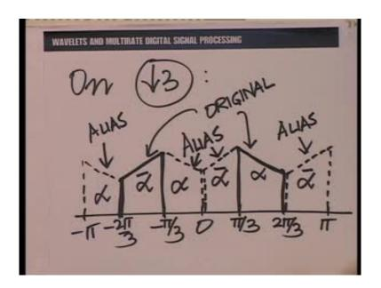
Now, as usual on down sampling by a factor of 3, we would be take this spectrum - this renal spectrum - after band pass filtering, shifting it by multiple of 2 pi by 3 and adding up the shift inverse; let me sketch what happens when we do so.
