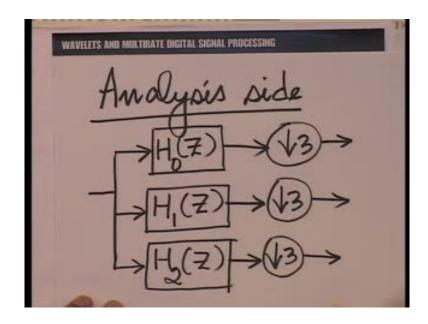
Essentially we have the same situation; we have 3 filters, that is called an H 0 Z, H 1 Z and H 2 Z, followed by a down sampling of 3, but this is true for any uniform 3 band filter bank; uniform actually refers the fact that, we have the same band, a band length of all the filters here.
