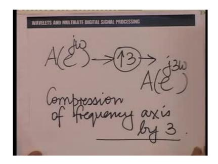
And if we look at the frequency domain for this, A inverse the power j omega is transformed on up sampling into e raise the power j 3 omega.
