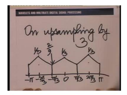
We go back here; so, you realize that an up sampling by 3, what is happening is a compression on the frequency access by a factor of 3. So, we see something very similar to what we had at the output of the down sampler, except that, there is a factor of 3 on the vertical axis; so, here we go.
