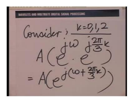
So, consider A e raise the power j omega times e raise times e raise the power j 2 pi by 3 times k is essentially a e raise the power j omega plus 2 pi by 3 times k, where k does not matters minus or plus, because anyway we are going to cover the three values 0, 1 and two modulo 3.
