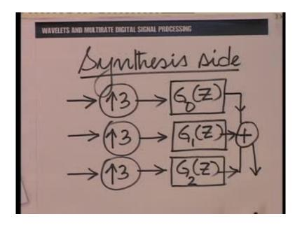
And on the synthesis side, we have in some sense, the transpose of the structure which would look like this; we have an up sampling by 3, followed by a filter and this is true for each of the branches.
