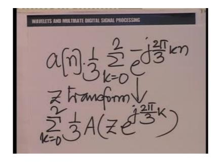
Then, a n times 1 third summation k going from 0 to 2 e raise the power minus j 2 pi by 3 times k n is going to have the Z transform, one third A Z e raise the power j 2 pi by 3 times k; that is easy to see some overall k.
