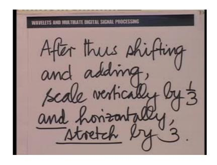
Now, multiplication by 1 by 3 here is a minor issue; it only means scale the spectrum by a factor of on the e by 3, but now the last step is to replace omega by omega by 3 and that is essentially an expansion step. So, what we are saying is, after thus shifting and adding, scale vertically by 3 rather by 1 third and horizontally stretch by a factor of 3, and that completes the frequency domain effect of down sampling by 3.
