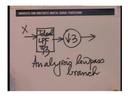
And we subject this spectrum to the low pass branch in the ideal three band filter bank. So, low pass branch is essentially low pass filter - ideal low pass filter - with the cut off of pi by 3, followed by a down sampler; and then, of course we have the analysis and synthesis side following the analysis side; this is the analysis side, but we will do the analysis of the synthesis side afterwards.
