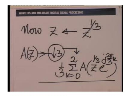
And of course, following that, what we are doing is to replace by Z by Z to the power 1 by 3; and therefore, when A in the Z domain is subjected to down sampling by 3, what we obtain is all and all, 1 third summation k going from 0 to 2 A z raise the 1 third times e raise the power j 2 pi by 3 times k.
