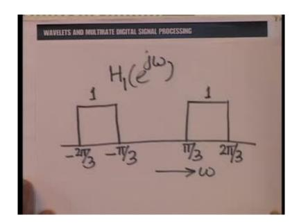
So, X 0 Z as the following ideal frequency responses, such you can see X 0 is an ideal low pass filter with the cut off of pi by 3. Now, H 1 is an ideal band pass filter between pi by 3 and 2 pi by 3.
