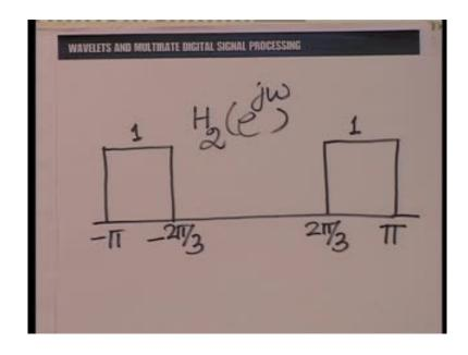
So, you could have a frequency response that looks like this. And finally, H 2 would be an ideally high pass filter with the cut off of 2 pi by 3. So, of course as we expect the 3 filters together H 0, H 1 and H 2, in some sense cover all of the frequency access from 0
