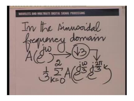
A very important result in it is own right and we need to interpret this in the frequency domain first, so in the frequency or in the sinusoidal frequency domain. So, in the sinusoidal frequency domain, A e raise the power j omega, when subjected to down
