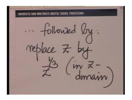
So, equivalent to multiplying by this followed by, replace Z by Z raise the power 1 third in the Z domain of course; what is what is meant by throwing away the zeros?
