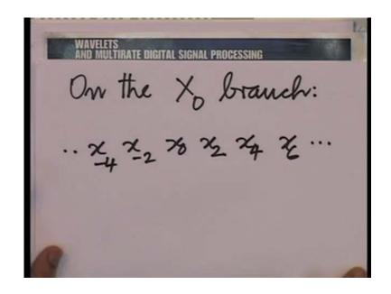
So, so let me right down graphically what I get on the x zero branch I get x zero followed by x two x four x six and. So, on this way x minus two x minus four and.
