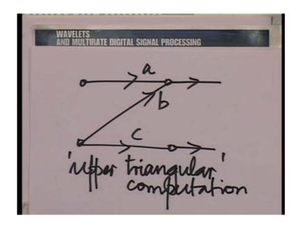
So, consider the upper triangular matrix let it have the form a b c as zero here what is the computation meant the computation meant is the following we are saying a upper branch is eight times this plus b times this the lower branch is just c times this. So, this is what is essentially a. So, called upper triangular computation and similarly we can put down a lower triangular computation.
