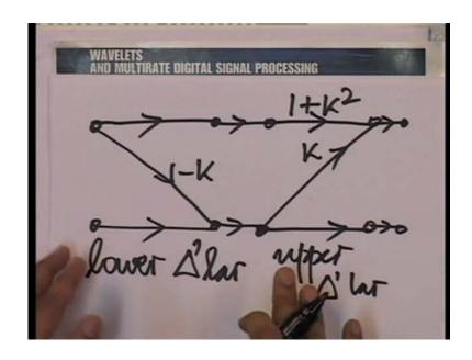
So, what we are saying in a fact is that one lattice stage computationally we have broken down this criss cross operation into a cascade of two operations. So, in the first operation we have one zero; obviously, this matrix operates first. So, one zero minus k one essentially meaning one zero is for the upper one this course as it is minus k one means minus k there and one here. So, the lower triangular part followed by the upper triangular
