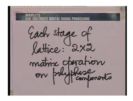
So, we could think of each stage of lattice as essentially a matrix the two cross two matrix operation on the polyphase components let us try and speak this language of matrices for example, when we simply delay the lower branch with the z inverse and leave the upper branch and change the corresponding matrix is essentially a diagonal matrix.
