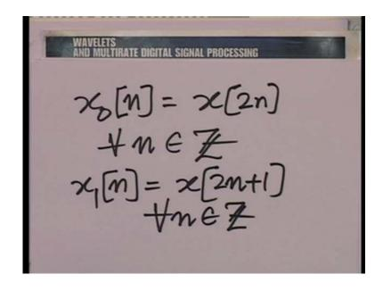
So, in other words we can define x zero n and x one n in terms of the sequence x n x zero n is simply x of two n for all integer n as we got x one n it is x of two n plus one for all integer n and it is very clear that x z
