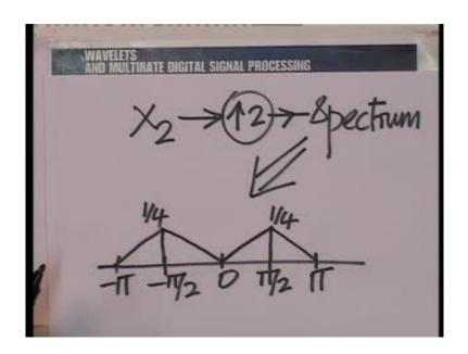
This also a factor of half, so this is the spectrum not of X 1, but of X 1 up sample by 2, so it is at this point that we have this spectrum, and now if you wish to construct the spectrum at this point all that you do is to invert the operation of the up sampler which you can do, the up sampler is invertible, so you just stretch this independent variable by a
