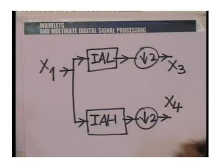
So, this input we shall call the point X 0 we will use capital letters, because we are going to work in the spectral domain all the while, we call the spectra X 1 and X 2 at these points, and we continue from here in naming the spectra. So, we have X 1 is further subjected to IAL and IAH with a down sampling by 2, here again and we get X 3 here and X 4, and the same thing is done to X 2.
