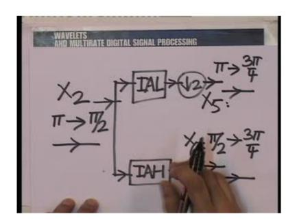
So, X 2 we are going to begin from pi by 2, from pi towards pi by 2 and when this is subjected to the action of the ideal analysis low pass and ideal analysis high pass followed by a down sampling by 2, what we are going to get here, is of course pi to 3 by pi by 4 without an inversion, but this already being one inversions, we have to bear with that.
