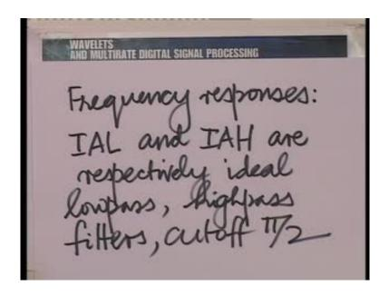
Let us first put down very clearly the frequency responses, IAL and IAH are respectively ideal low pass and high pass filters discrete time filters of course with cut off pi by 2, and therefore it is very easy to write down the spectrum at X 1 and X 2, you see let me put back those 2 before you.
