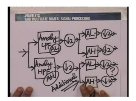
Now, the next time we take this entire structure and put it here, so we have a structure like this, let me call this analysis low pass filter as AL, and let me call this AH the analysis high pass filter, what I am saying is we put AL here and AH there, and this is what gives us the discrete wavelet transform, so this part constitutes a discrete wavelet transform, of course with this down sampled and left where it is.
