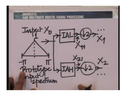
So, if we take X 1 here we have to input X 0 subjected to low pass filtering, that means the spectrum between 0 and pi by 2 is going to get extracted, we have done this before so I am not repeating all the details, so if you wish may be for simplicity what we could do,
