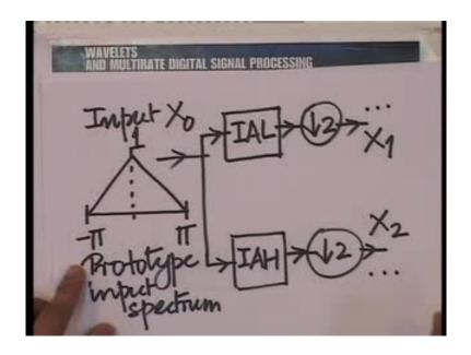
So, we take X 2 subjected to the operation of IAL, IAH down sample by 2, and obtain X 5 and X 6, and we wish to study the spectra of X 5 X 6 X 3 X 4 X 2 and X 1. Let us go about this task. Now, X 1 and X 2 are very easy, in fact we can write down the spectra in just one step.
