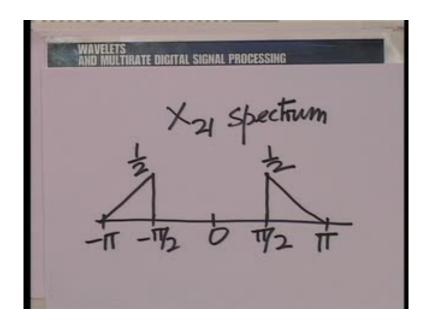
So, X 1 1 is very easy X 1 1 is going to have a spectrum like this, after all X 1 1 is obtained by subjecting the input to an ideal low pass filter with a cut off of pi by 2 that is very easy to determine. So, this is the spectrum at X 1 1, and similarly the spectrum at X 2 1.
