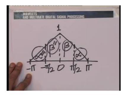
So, in fact let us mark out the spectral segments of the original spectrum, let us call this spectrum, of this segment of the spectrum alpha, and this segment shall correspondingly be called alpha prime or alpha double dash if you like, we call this beta, and we call this beta double dash here.
