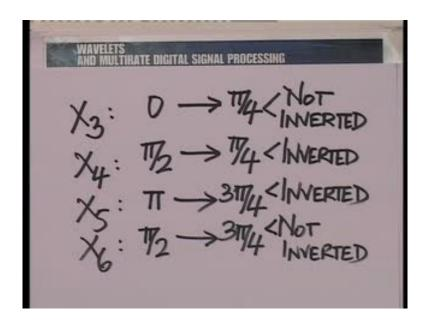
Anyway, let us write down these results very clearly, so what we are saying in effect is, X 3 is essentially the components from 0 to pi by 4 not inverted, X 4 is the components from pi by 2 to pi by 4 inverted, X 5 is the components from pi to 3 pi by 4 and inverted, and X 6 is the components from pi by 2 to 3 pi by 4 not inverted.
