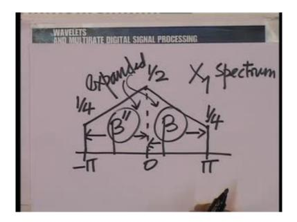
On a similar note if you look at the spectrum of X 1, this part of the spectrum here, between 0 and pi is actually the spectrum beta, so this is beta here. And beta double prime from the original spectrum has found its place here. Of course they are again expanded as before.
