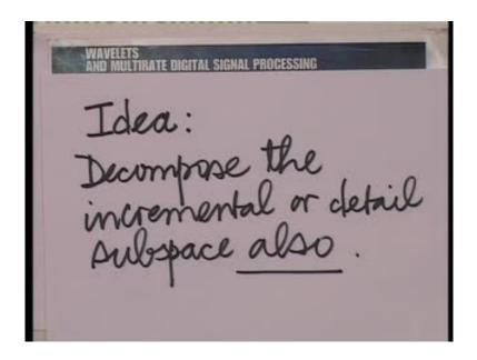
In the wave packet transform or objective is to get around this limitation, so what we intent to do, is to decompose the incremental sub space as we do the approximation sub space, so for example when we decompose V 1 into V 0 and W 0, we also intent to decompose W 0 in the next step or if you go one step higher.
