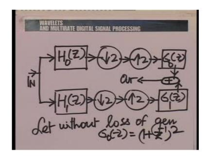
So, let us consider a filter bank, a two band filter bank. Just to recaptulates some of our ideas, what we are saying is we have this two band filter bank, where the low pass filters are h 0 z and g 0 z on the analysis and synthesis sides respectively and the high pass filters are h 1 z and g 1 z, again on the analysis and the synthesis sides respectively, in here, out there.
