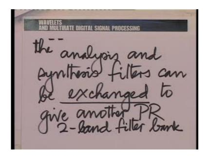
Once the perfect reconstruction conditions are satisfied in a 2 band filter bank, the analysis and synthesis filters can be exchanged to give another perfect, the p r stands for perfect reconstruction, perfect reconstruction two band filter bank.
