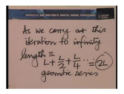
So, you can see that the length is not going to go to infinity but it is going to converge, and what is it going to converge to very simple. As we carry out this iteration to infinity, the length is going to converge to 1 plus 1 by two plus 1 by four and so on. It is a geometric series and the sum is very easy to calculate its two l.
