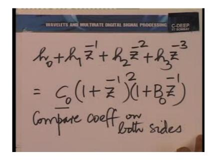
So, all that you have is h zero h two plus h one h three is equal to zero. This is the only nontrivial equation that we get. Now, from the location of the zeros and the free parameter, we need to express h zero through h three in terms of the free parameter. So,
