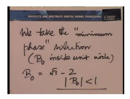
So, when we take the solution inside the unit circle, we are reducing the phase or the group delay as much as we can in the filter. So, it is essentially a question of choosing the better solution in terms of phase. So, let us summarize that. We take the minimum phase solution, that is, b zero inside unit circle and we have b zero is square root three
