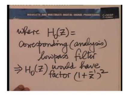
The high pass filter would have a factor of one minus z inverse the whole squared, and therefore, if we look at the low pass filter, remember, the high pass filter was essentially of the form z rise the power minus d h zero minus z inverse, where h zero z is that corresponding low pass filter, of course, I am talking about the analysis sight.
