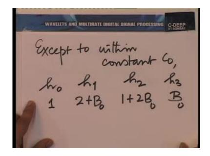
Anyway, we can now put down the impulse response of the daubechies low pass filter. Therefore, it is essentially, well, let me read of the impulse response from here. Let me flash the impulse response before you once again, and then, will substitute. This was the impulse response, now, we substitute for b zero.
