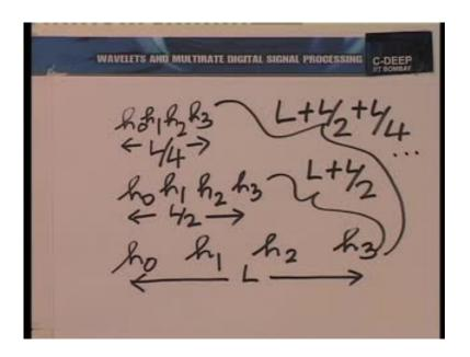
So, what I am saying is it is a convolution something like this. You start with a train of impulses which is spread over a length of l. The next time, the same train is squeezed by a factor of two. So, its spreads over a interval of l by two. The next time, it is squeezed
