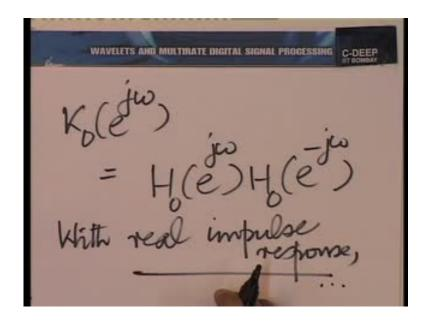
So, what we have is essentially the following equation. The principle equation governing the quadrature filter bank is this - kappa zero z plus kappa zero minus z is a constant, where kappa zero z is h zero z h zero z inverse, and therefore, if you look at it the frequency domain says kappa zero e rise the power j omega is h zero e rise the power j omega h zero e rise the power minus j omega essentially.
