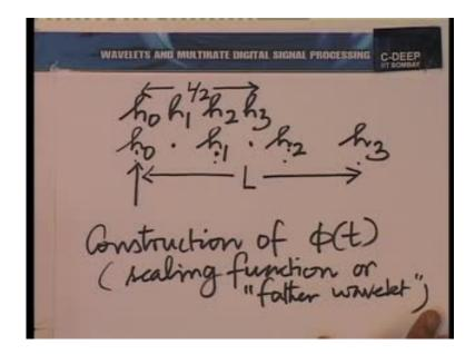
So, essentially you would have a situation where you first construct h zero h one h two h three lying on, you know, so the situation is that you need to compress and convolve, compress and convolve, as we did in the haar cases well. So, you would start essentially by putting h zero h one h two h three like this. Then now, now remember, what we are doing here is to construct pi t the scaling function or the so called father wavelet.
