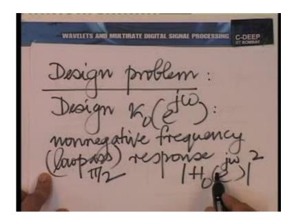
So, you know, this equation that we had here kappa zero z plus kappa zero minus z is a constant. Essentially says the even samples, other than the zeroth sample is all zero. So, you are trying to design a low pass filter. So, in fact, we should qualified this further non negative low pass frequency response, and what kind of a low pass frequency response with a cut off pi by two. Now, we have the design problem very clear.
