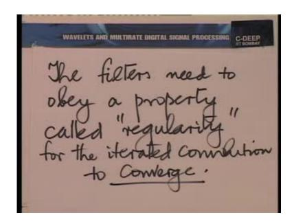
There is no such guarantee that any such arbitrary filter would converge in this iterated convolution. So, what is it about this filter which allows convergence? In the literature on wavelets, they speak of this as a property called regularity. So, we say that the filters need to obey for the iterated convolution to converge. Converge to what? Well, converge
