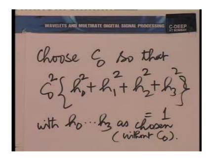
So, now, we shall choose c zero in order that this becomes one, and in fact, I no need to carry out the computations. Essentially what I am saying is choose c zero so that c zero squared times h zero squared plus h one squared plus h two squared plus h three squared is equal to one with h zero through h three as chosen before without c zero.
