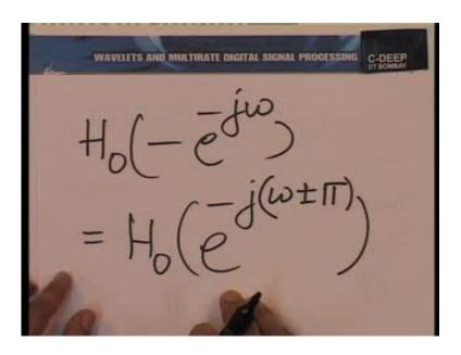
So, we said this minus essentially shifts by pi, and therefore H 0 e raise the power minus j omega without the minus sign would have been a low pass filter as it is, because of this conjugate symmetry that we have here, and now with the introduction of a minus sign, it becomes a high pass filter. So we have a convincing argument now that H 1 Z, the way we have constructed it.
