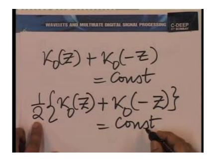
This gives us a sequence corresponding to the inverse Z transform of a constant, which is essentially an impulse. Now, you know this modulation is what we derived when we talked about the Z transform across a down sampler.
