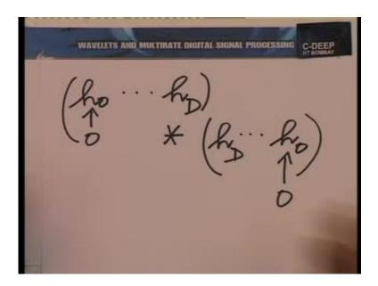
Now, H 0 Z times H 0 Z inverse corresponds to their convolution, you know when you multiply to Z transform, the corresponding sequences are convolved, and therefore we have this convolved with this, maybe I should put parenthesis here, and indicate the 0 clearly there.
