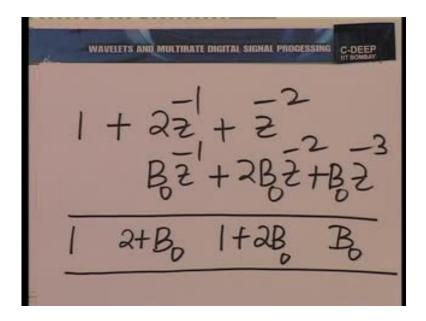
That product will be 1 plus 2 Z inverse, plus Z raise the power minus 2, plus B 0 Z inverse times this, so B 0 Z inverse plus 2 B 0 Z raise the power minus 2. plus B 0 Z raise the power minus 3.
