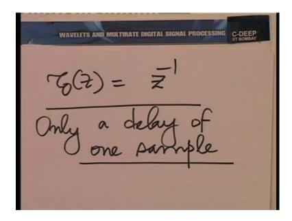
So, the tau 0 z, all in all is z inverse. What is this mean essentially? Only a delay of one sample. The constants have already been accommodated. So, . So, c 0 becomes 1. Now, why was this delay required? As i said, this delay is required on a count of causality. If we did not want this delay to be there, we would need non-causality either on the analysis or in the synthesis side.
