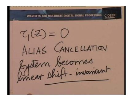
You know, when there is an alias term, the words "system function" is actually a misnomer. One should not use the term system function because the system is not linear and shift-invariant. On the other hand, if tau 1 z is 0 the system becomes linear and shift-invariant.
