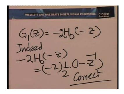
G 1 z in the haar case should then be minus H 0 of minus z or rather with a factor of 2; so, two times. And, indeed minus 2 times H 0 minus z is minus 2 times half into 1 minus z inverse, which is correct. So, things have all fallen into place. It is convenient.
