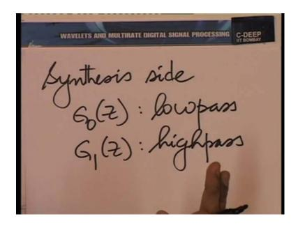
Synthesis side: G 0 z, low pass filter; G 1 z, high pass filter. So, this is the circumstance. Of course, you know where the down samplers and up samplers are. The relation between Y z and X z is as follows.
