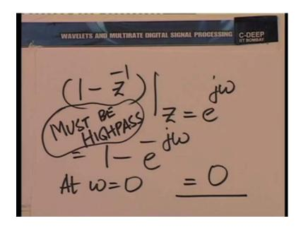
So, in other words, in a certain sense, the more 1 minus z inverse terms you have and by the way, we soon see these terms are going to be on the high pass branch; is not on the low pass branch. You know 1 minus z inverse, when we substitute z equal to e raised to the power of j omega, vanishes at omega equal to 0. It is verified.
