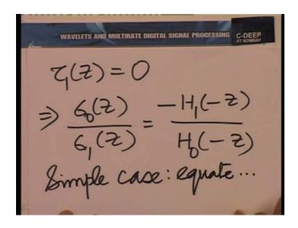
And, tau 1 z equal to 0 means essentially that G 0 z by G 1 z must be minus H 1 of minus z divided by H 0 of minus z. And, the simple case is, equate the numerator and denominator.
