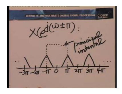
Would therefore, appear like this. Again, we shall do a bit of zooming here and so on here and so on there. So, now here triangles are around pi and then 3 pi and so on and here around minus pi and then minus 3 pi and so on. So, now again if you take the principle interval which is here, this is what we get.
