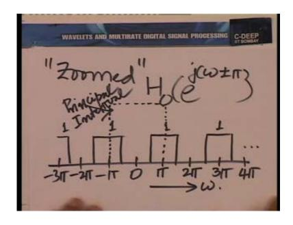
It would have an appearance like this and so on here. This pass band so to speak and now going to lie at odd multiples of pi and you can continue that drawing. Now once again, we confine to the principle interval, the principle interval is here.
