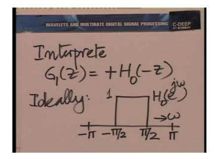
You see ideally this is what the frequency response of H 0 Z should be, it should be an ideal low pass filter with a cutoff of pi by 2. So, this is what the frequency response should look like. This is 1 the height here. So, what would H 0 e raise the power omega j omega plus minus pi look like. In other words, what is H 0 of minus Z then?
