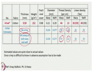
With these two assumptions, if we proceed further, it is observed that the actual values are provided in the first row of the table. For the cotton fabric, the thickness, weight, fractional cover, and diameters of the warp and weft are all given. The thread densities (warp and weft) and the linear densities of both yarns (warp and weft) are also stated. These are the actual values used in the construction of this fabric.
