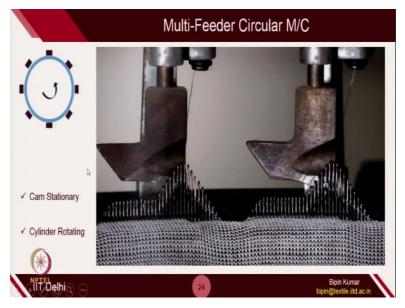
So, let's see how it works. So, you can here there is another video here, actual running of the fabric on this machine. (Video Starts: 43:58) So, the needle is revolving, so you can see here, the needle is revolving. So, needle is first making loops interaction with the cam placed here. Once this needle make the loop here, it is carrying and interacting with the second cam in the same circle.
