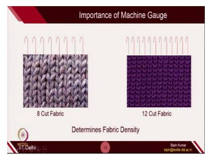
Why this machine gauge is so important? Because, depending on what type of machines you are using for the fabric production the fabric quality or fabric density will be decided. For example: Here, this is 8 cut fabric, so here you can see; for making 8 wales, 1, 2, 3, 4, 5, 6, 7, 8. So, 8 needles was used in the same area. But for the same area, you can see here, in 12 cut fabric, 12 needles was used for the same width of the machine.
