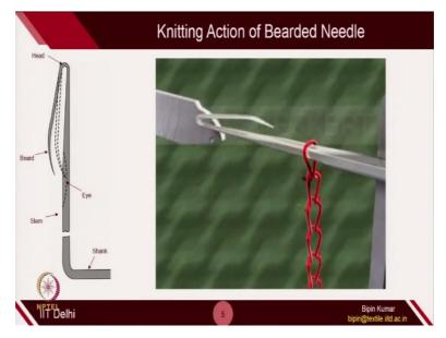
Now, move to the beard needle; how the knitting action is possible with the help of beard needle. So, in, if you see the structure of beard needle, it is not look like a latch. It has the head part similar to latch needle, but it do not have latch, but it has the beard. Okay. So, you can see here, this is the beard part and this beard part is flexible. Okay. So, this beard part can go inside the slot. And this slot is eye.
