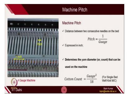
It is actually the distance between 2 consecutive needles on the bed. So, you see, the needles are placed on the bed. And distance between 2 consecutive needles is called pitch. So, if you calculate the distance; here you can see, in 1 inch, there are 4 needles are placed. So, distance between 2 needles naturally will become 1 by 4. So, there is a small relation where pitch is actually one by gauge.
