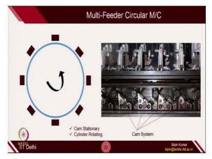
In case of single feeder, only one cam was there and the feeder was also moving with the cam. But in case of multi-feeder machines, many cams was located along the circumference. So, if you see the actual photo, so here these cams are placed on the cylinders. So, across this curved part of this cylinder, many small small cams was placed. So, these are all cam system that is placed on the cylinder.
