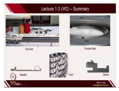
So, the first thing we started in this week was automation of loop formation. So, I introduced to you the importance of needle and how the needle was responsible for making loops. Needle interacts with the cam and it follows the path of cam which was created by multiple cams by placing in a certain sequence. And the needle butt actually follows the path of this cam track, due to which it continues its loop formation process.
