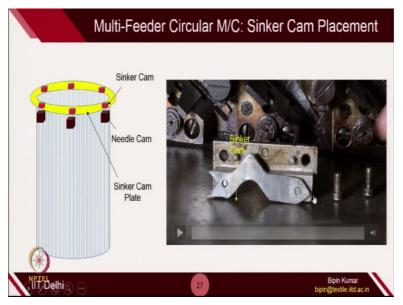
Now, let's see how the sinker is placed. So, if you try to observe, there is a sinker elements is also there on the machine. So, needle cam is placed on the cylinder's curved section and which is stationary and cylinder is rotating. The sinker cam is placed in this plate. So, this is the plate on which sinker cam is placed. So, these 2 cams works together at the time of knitting loop. So, I am showing you how the sinker is placed.
