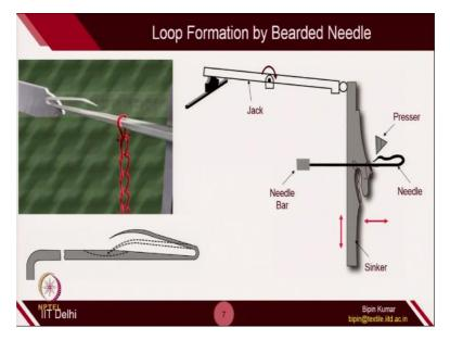
If you see the machine, so the machine looks like this. So, apart from this beard needle, it has 2 segments. One is the sinker part and the another one is the pressure part. If you now see carefully this animation, (Video Starts: 13:32) it is the sinker part which is taking the loop inside the beard segment. Okay. If you see again, this is the sinker part which is taking the loop inside the beard part and also making the sinker segments.
