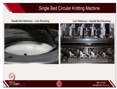
The other way we can divide this circular knitting machine is, how the rotation is taking place. So, in first case, the cam is rotating but the needle is just doing reciprocating movement in the same vertical line. Okay. So, the needle is not rotating on the curved surface, rather cam is rotating. So, let's see this video. (Video Starts: 36:42) So, here you can see, this cam plate, this is rotating.
