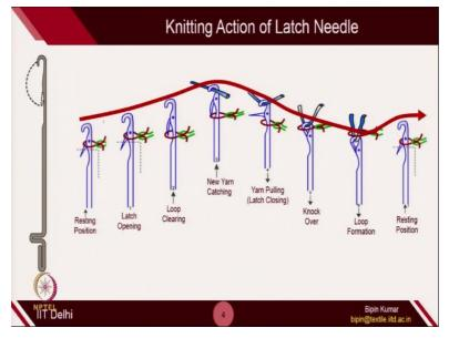
Just a quick recap, we have already introduced you how the reciprocative movement of needle was done with the help of cam track. So, okay, the butt was engaged with the cam track. And because of this, certain sequence was followed by the needle. And due to this sequence, it was forming the loop. So, it started with the latch opening, because the needle starts raising. And then, the loop was cleared.
