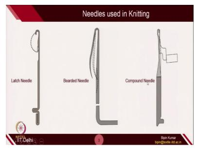
Latch needles, the main important part is the latch itself. That's why this needle is named latch needle. Latch is actually helping in closing the hook and opening the hook. And this action of opening and closing of latch, is self-sustained, because we don't need additional motor or motions to open or close this latch. We have seen already, how the latch is opened by the yarn itself.
