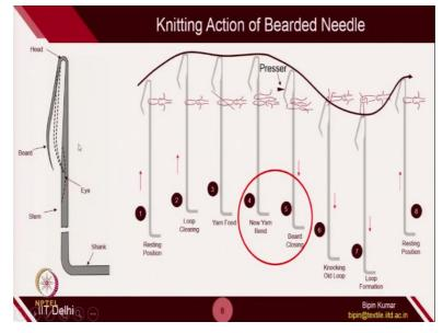
Similar to latch needle, the reciprocation has to be done, but in a certain fashion. We again have the resting position similar to latch needle where it is holding the old loop. Okay. So, the first thing, to catch a new loop or new yarn, this old loop has to come out from the beard and head segment. Okay. So, this head and beard segments, this old loop has to come out. To do so, there is a step of loop clearing in which this particular needle raises upward.
