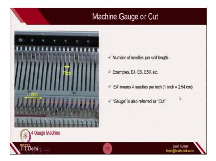
So, machine gauge in simply it is defined as number of needles per unit length. So, you have seen how the needle was placed on the trick or the slot inside the bed. So, here is this bed. And in each of these slot, a needle is placed. So, this is the butt segment of the needle and they are placed on the bed. Naturally the placement of these slots can be made very very finer, depending on what type of tooling machines you are using.
