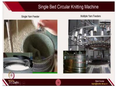
So, in one case single yarn feeder. So, you can see here, this is only one yarn is being used during knitting. But in case of multi-feeder yarn, you can see so many yarn bobbins are placed on the top of the machine. And at the same rotation, all of these yarn ends are used inside this cylinder. In industry, mostly it depends on the, how fast you can produce the fabric.
