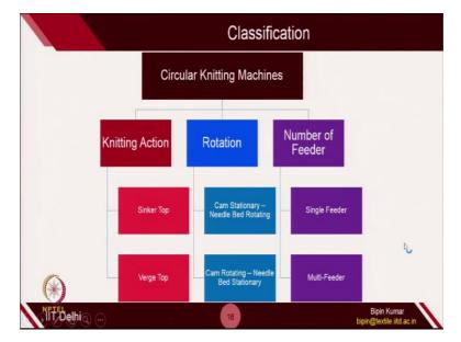
When you see circular knitting machines, it can be divided into by 3 categories, by knitting actions which I already covered in the last class. The classification is done by sinker top and verge top machines. Rotation: so, how the rotation is done on the circular machine. It can be further categorized by 2 ways. One is cam stationery and needle bed rotating. So, here the cam is stationery and needle is rotating and the butt is interacting with stationary cam.
