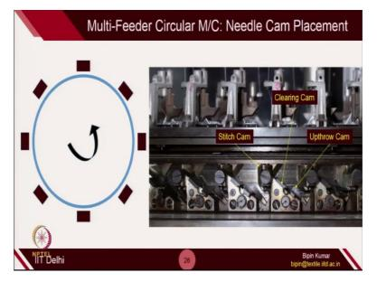
Now, let's try to observe the needle cam profile. So, each of these cams which is placed along the circumference, they do the same, some kind of reciprocative movements to the needle butt to make the knitting happening. (Video Starts: 44:43) And is a small video you can see here. So, the needle butt first interacts here. And it starts rising. Then again it hits this particular cam, then it rise.
