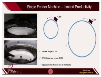
So, if you see single feeder machines from lecture 3, the cam was rotating and this was the cam. (Video Starts: 38:47) If you see this, the cam was rotating and the fabric was formed. Then you can see this vertical yarn which was feed in the fabric forming zone. Okay. And if you see, if you slow down this process, what you can realize is, whenever the cam is interacting you can see the needle is either raising or the sinker is going inside, depending on the position of the butt.
