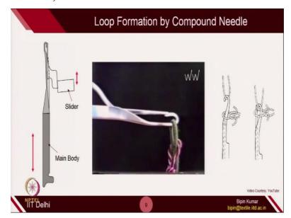
Here is a another small video from YouTube which you can see and observe how the loop formation was done. So, initially the old loop is on the stem segment and the latch or the slider part is inside. So, this slider part is inside the slot of this main body. So, you can see here, it is inside the slot. Once the head part of the needle, from the main body; this is the head part. This head part catches the yarn.
