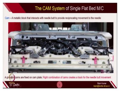
So, if you reverse the cam jacket, it will look like this. So, this is the back side view of the cam jacket. At this moment, it looks very complicated. You can easily see, it consists of lot of metallic raised blocks. And these blocks are placed in a specific order. And at this moment you would not be able to understand what was the track the needle was following. But let's have a look to this particular cam track in detail.
