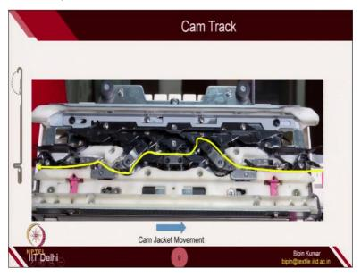
If you reverse the path, the same nature of movement is observed. (Video Starts: 15:08) So, you can see here, again the butt is going, then coming down, then down; and then finally it come to original position. (Video Ends: 15:17) This time, the cam jacket movement was from left to right. And with respect to cam jacket, the needle was moving towards left. While in the previous slides, the needle was moving towards right and the cam was moving from
