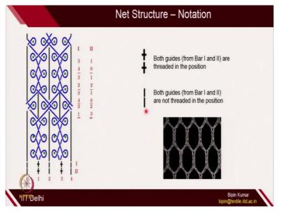
In reality, you have a different way of denoting the net structure. So, in net structure, actually you need to find out, not only you have to describe the position of guides, but also you have to explain which guides is carrying the yarn and which is not. So, plus plus, both guides from bar 1 and bar 2 are threaded in this position. So, for example, if you see this figure. So, first position and third position, both the guides are carrying the yarn.
