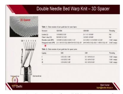
So, in 3D spacer structure also, there are lot of possibilities. You can go for 6 guide bar which is most popular. So, let me show you one simple structure of spacer. (Video Starts: 34:24) So, now you can see, this is the spacer structure. So, they are 2 layers. So, one is, this one is front layer. Okay. And the other one is the back layer. And they are actually connected with connecting yarn.
