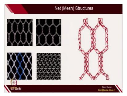
So, in net structure, if you see, is basically we call these type of a structure as a mesh structure. So, you will create a different kind of meshes or holes in the fabric structure. This was the highly dense loops and this is the more porous one. This one is also, it looks like a rhombus. This looks like a hexagonal. So, here also, the schematic if you see, this looks like a perfect hexagonal structure. So, how do we actually create these type of structures?
