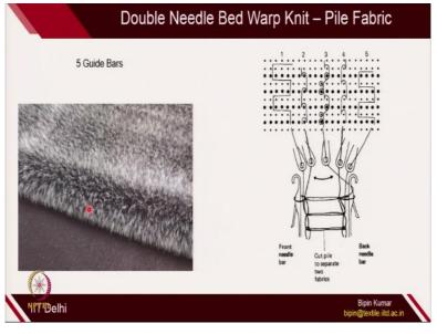
Similarly, you can have 5 guide bar structure. So, here also, you can see 5 guide bar structure. So, there are 5 guides, 2 beds. So, 2 guides is focusing only on making fabric development with the first bed. And 2 other guides is making only fabric with the back bed. And there is 1 connecting bar. So, again if you follow the bigger dot and smaller dot. So, the guide number 1 is just doing underlap on front bed.
