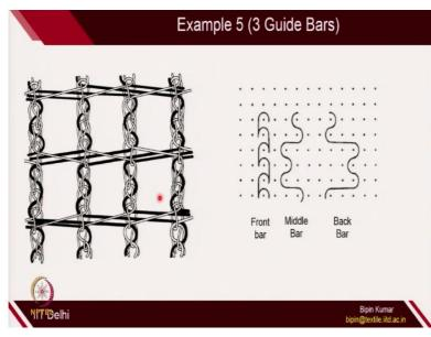
Even you go for more complicated one. So, here the front one is making pillar. And middle and back one, other 2 guides are doing inlays. So, here also you can generate very uniform mesh structure. So, this is another alternative way. You can use the inlays selectively to create mesh pattern.
