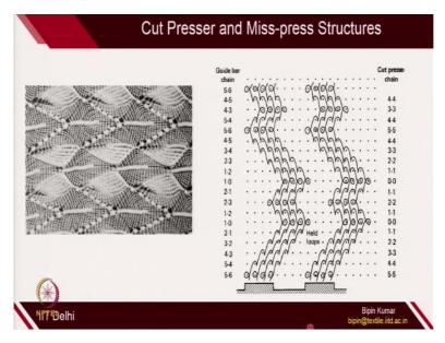
So, for example, if you want to create this structure; so, you are doing the lapping of some of the guide bars, while the other guide bars is holding the loops. Okay. So, this needle is hold the loops for 5 courses. And because of that, some opening is being created. So, somewhere, you have more dense areas, because more loops are being generated. And wherever you have more held loops, there the structure is more open.
