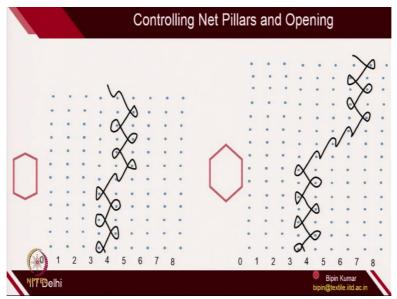
So, for example, if you see this particular, a simple example, just to give you a hint, how you can change the dimension of this mesh. So, here is the lapping position of both the guides. And in one case you are doing tricot for 5 courses. And then, you are doing the transition. You are just doing 1 transition with the help of 1 open loop. And then, again you are doing 5 course of tricot.
