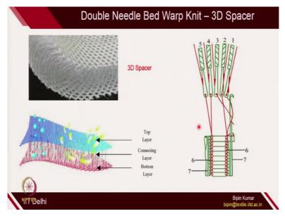
The other important structure is 3D spacer structure. So, 3D spacer structure is again, you are making 2 fabrics on 2 different beds. And there will be 1 connecting guide which is connecting both the fabric layers. So, there is top layer and bottom layers. And these are connecting layers, which is called spacer yarn. So, here also, if you see the 5 guide bar is there.
