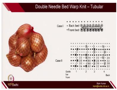
The last one is the tubular fabrics. So, this is the tubular fabric. So, here also, you need 2 beds. So, 2 fabrics layers will be created on each of the bed. And from the ends, there will be 2 guide bars which will be connecting just these 2 structures. So, here you can see. So, on one side, you are making 1 cross 1 tricot on the front bed. And the other side also, you are making 1 cross 1 tricot on the back bed.
