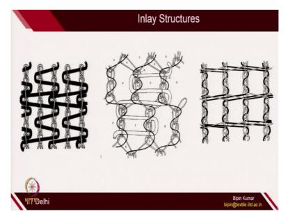
So, inlay structure is like, here the yarns are actually floating in the fabric structure. (**Refer Slide Time: 21:19**)
