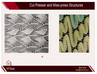
So, as you have seen in warp knitted, the loop geometry is highly, highly complicated, because the positioning of underlaps which is not providing equal tension to the each loops. So, because of that, you will get a different kind of pattern. And including with such a complicated underlaps, if you can play with the held loop, tuck loop or miss loop, you can get even more complicated structure.
