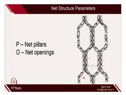
So, net structure parameters. There are 2 main parameters in net structure. One is the pillars, the vertical line of the mesh. And the O is the net opening. So, what is the distance between 2 vertical pillars. And the other sides are just the transition of guide bar from one pillar to next pillar.
