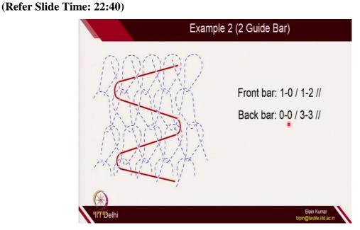
The second one is also 2 guide bar structure. Here, front one is making tricot 1, 0, 1, 2. And back bar is just doing underlap, no overlap. So, here they are 0, 0, no overlap; 0 to 3, underlap.
