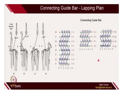
So, in double bed structures, naturally there are 2 beds and multiple guides, guide bar. So, now the onus is on the guide bar, to switching from one bed to other bed. So, if you see this guide. So, first it is making loops in the front bed. After making loops with the front bed, it is moving to the back bed. So, when it is moving loops with the back bed, the front is resting. When it is making loop with the front bed, the back bed needles are resting.
