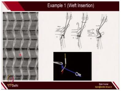
For creating inlay structure, the most easy way is the weft insertion. So, once the guide bar is at the back position, you can carry the yarn and put it at the back side of the needle. So, this is how (**Video Starts: 21:32**) you do the inlay. So, you put the weft yarn at the back side of the needle. And then, you are doing the overlap and underlap. So, because of overlap, the weft yarn is locked between the loops.
