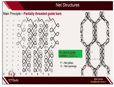
So, to create these type of structures, we do need only 2 guide bar on the machine. Just like front and guide bar for locknit or sharkskin. The machine will remain same, only what we need to do is the, we need to thread the guide bars selectively. So, in a regular warp knit structure where all the guides of each bars were filled with the warp yarns, but in case of net structures, we have to leave some guides empty.
