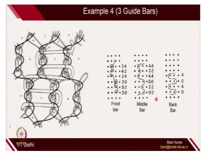
Similarly, even more complicated structures can be generated. So here, this is the front one. And the middle one is just doing the inlays. And back one is also doing inlays in a different way. It made from 3 guide bars.
