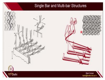
So, this is the single and multi-bar structure. I have already introduced you how we can denote this single bar structure. And this is the double bar structure. Just I showed you. So, single bar and multi-bar structure is like when you are using only one set of guides, which is in, attached with 1 guide bar. Then, it is a single guide bar structure. So, at a same time, only one guide is providing yarn to the needle in each course.
