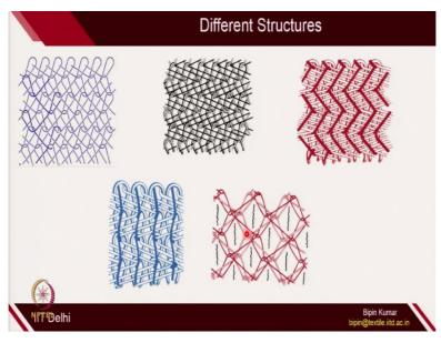
So, some of the structures I already mentioned; single bar structure, double bar structure. This is also double bar structure. This is also double bar structures. This is also double bar structure. So, from technology point of view, how technology actually helps in designing different structures.
