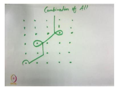
So, I am just giving you hint; combining all, combination of all. So, for example, let's suppose I am doing this. So, here you can see the overlap and underlap are in the same direction. Here you can see overlap from right to left; and underlap, left to right. Here, you can see only floating yarns. So, each course has the combination of different arrangement for overlap and underlap.
