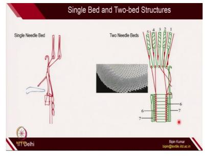
So, in single bed, here only one set of the needles are attached with 1 bed. And different guides are providing yarn to that particular needle bed. But sometimes, 2 needle beds can also be fixed, facing opposite to each other. So, this is the first needle bed; and this is the second needle bed. And you can see all the guides are playing across these 2 needle beds and creating different types of warp knitted structure.
