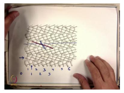
So, the first thing before you move on. You need to find out what is the movement pattern for each guide bar. So, this is a 2 guide bar structure. And how do you find whether it is a 2 guide bar or single guide bar? Between 2 loops, you can find how many floating yarns are there. Okay. So, if you carefully see, between these 2 loops, any 2 loops. So, let's suppose if I am following these 2 loops; so, between these 2 loops, you can see there are 2 floating yarns in different directions.
