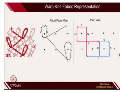
So, to represent a fabric, you need to first go for microscopic view, get the real picture of the fabric. And then, you start following one individual yarns. Because, based on the basic features, if it is having just 1 guide bar fabric, then you can extract the movement of 1 individual yarn. So, this is the actual fabric view where the loops have been created by one individual needle.
