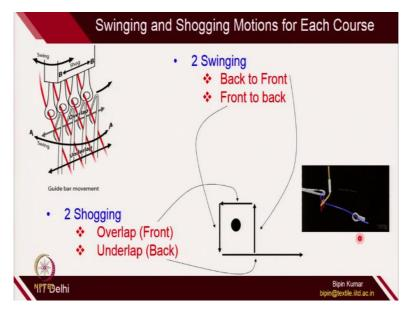
So, swinging and shogging motion is done by the guide bar. And one guide bar consists of many, many guides. And each guides provides yarn to 1 particular needles. So, in the last class, with the help of animation, I showed you what are swinging motions and what are shogging motions. So, swinging motions, I discussed, like the guide bar is moving from back side of needle to front side of the needle; as well as, the guide bar is moving from front side of the needles.
