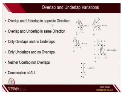
The other, last important design principle is, playing with overlap and underlap. So, I have already told you; overlap and underlap is required during each course formation. So, and these pattern of overlap and underlap has different possibilities. So, for example, you can go for overlap and underlap in opposite direction. So, you can also go for overlap and underlap in same direction.
