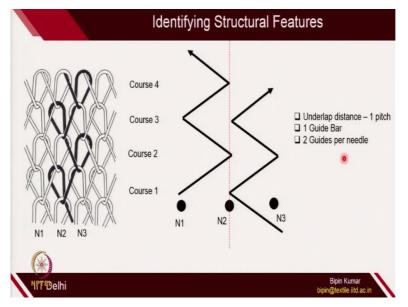
If this thing is clear to you, you would be able to first identify some of the features of any warp knitted structures. For example, how the guide bar is switching from one column to other column; what is the nature of shift; how many guides are actually interacting with individual needles during the fabric formations; how many guide bars are there. So, all those important features, you can extract by looking to the microscopic view of the fabric.
