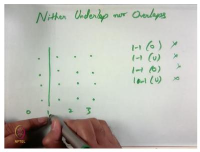
And the last part, neither underlap nor overlaps; nothing is happening. So, if nothing is happening, 0, 1, 2, 3; it means, the yarn is moving completely in a straight fashion in every courses. So, if you see here, we have 1 to 1 is overlap; 1 to 1 is underlap; 1 to 1 is overlap; again 1 to 1 is underlap. So, there is no movement at all. So, the yarn is being provided. The guide bar remains in the same position carrying the same yarn between these 2 needles. Okay.
