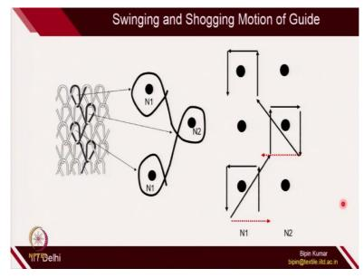
So, further, I tried to explain the fabric with some kind of lapping diagram and some kind of lapping plan, because instead of drawing this so complicated diagrams, we can simply draw the movement of one individual yarns. And we can denote their movement by some numbers. You can see it here. So, first, the loop is being formed by N1 needle. And then, in the second course, the loop is being formed by N2 needle for the same yarn.
