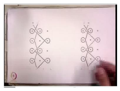
For example if this is a 2 bar structure, second guide bar is switching from first needle to second needle and if you see the first guide bar it is switching from third needle to first needle ok. So you can just write down this lapping diagram here, so here you can see this is the lapping plan, so for each guide bar you can write down this lapping plan. So for guide number 1 and guide number 2, similarly here also there are 2 different guide bars.
