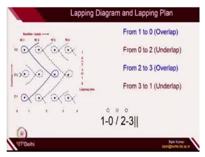
So if you see carefully the lapping diagram, that lapping diagram can be expressed by certain numbers which is called lapping plan. So following the movement of this particular position of guide, it is first swinging then shogging then going back and then again shogging. So this is what the guide is doing first from 1 to 0, so basically it is moving from 1 position to 0 position and providing the yarn, so this is nothing but overlap.
