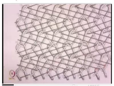
So if you see here one yarn is switching from one column to other column and the black one is switching from one column to fourth column. You need to collect all the informations in one place and then you need to design the lapping diagram for each guides. And in this way you can represent this fabric structure, more practice we will do in the next class so at this moment I think this is more than sufficient.
