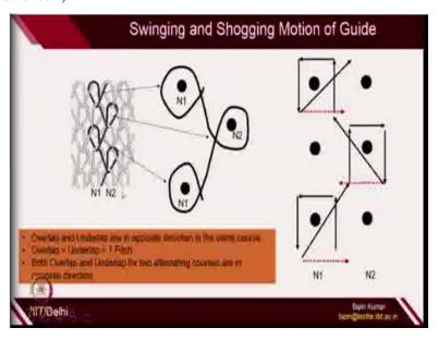
This is the swinging and shogging motion for this particular simple structure. So first the guide is coming to needle N1 then guide is for making the loop it follows 1 swinging then shogging front side, then swinging then shogging backside. So these 4 numbers we have to explain and after that it is moving to N2 and it again make the loop again swinging shogging, swinging shogging.
