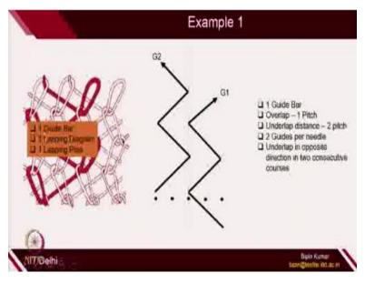
So 1 guide bar fabric, so we need 1 lapping diagram for 1 guide bar and 1 lapping plans so 4 digit numbers ok .
