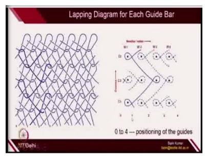
So this is what we have to explain, so this fabric can be represented by simple lapping diagram of each guide. So to describe the lapping diagram of each guide we have to first denote some numbers or some starting position which is expressed here. So on the left side of this column the position is 0, after first column the distance between these 2 columns are represented by number 1.
