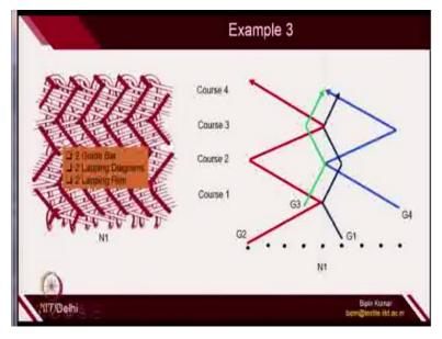
Similarly if you see this structure again a 2 bar structure, so 2 lapping diagrams and 2 lapping plan is needed to describe this fabric structures.
