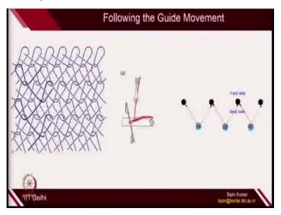
Let me show you some examples, for example if you see this particularly structures and carefully you can follow one of the movement of yarn. So if you see the dark one you can start from here it is first making loop this way then it is moving to the first column making loop. Then it is again
