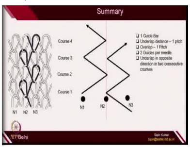
In the last class I also mentioned how the needles was interacting with different guides during loop formation. And for example this structure all the guides have the same movement, so they can be attached with the same guide bar. We have the underlap distance of one pitch, overlap distance in the front side is also for one pitch. We have 2 guides per needle because you can see in alternating courses the guides are changing for needle number 2, so they are 2 guides.
