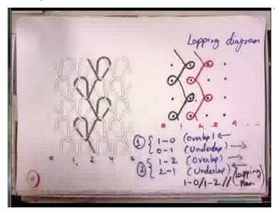
So this is the lapping diagram and lapping plan, now let's look at this particular fabric because we are looking at this fabric multiple times. So let's see how do we start, the first thing we need to denote the position, so the first position is 0 position, then second position, third position, fourth position, fifth position. So 0 indicate the first position of guide bar, first indicate the second position of guide bar, 2 indicates third position of guide bar.
