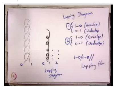
We can have more complicated also, for example this is another fabric having just providing yarn to the same column. So here if you follow the path of the yarn it is just providing yarn in the same needle, it is just providing yarn to the same needle. So if we follow the path of the yarn it is providing yarn to the same needle ok, so again you can write down 0 and 1, so 0, 1 then 2 position, so this is the lapping diagram and for this particular guide how the things will be moving.
