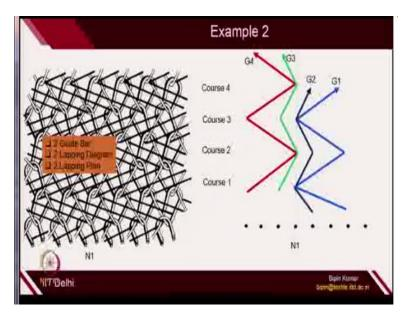
If you see this particular fabric, so you have 2 guide bar because we explained in the last class also. So for each guide bar we need to have 1 separate lapping diagram and for that lapping diagram I need to have separate lapping plans. So for describing this fabric I need to create 2 lapping diagram and 2 lapping plan.
