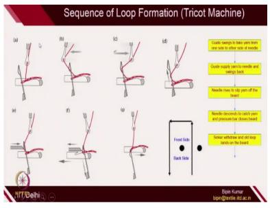
So sequence of loop formation on tricot machine. So as I mentioned for making a loop in a warp knit structure you need 3 elements one is needle, one guide to supply yarn and sinker to help in loop formation. So these 3 elements is a must. So before the formation of loop formation the guide is actually standing at the backside of the needle. So if this is the needle and if you are assuming the front side on the left side of this figure.
