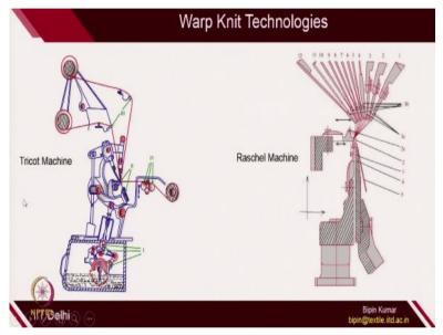
So in the market there will be 2 type of technologies which you will find out in warp knitting. First one is Tricot machine and the second one is Raschel machines. The name is just the name, but ideally speaking the principle of loop formation remains same there will be interaction of needle and guide in both the machines.
