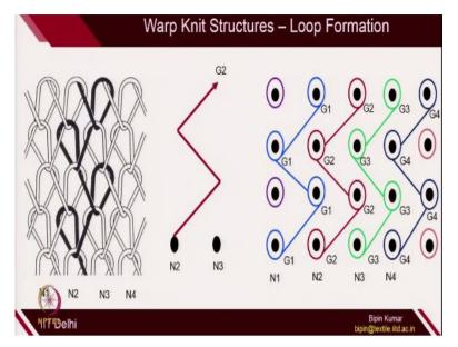
So again I showed you how the role of guides and needles are important in loop formation. For example, here in the first course needle N2 is making loop using the yarn from G2. In second course the G1 guide is providing loop to needle N2, in third course again G2 guide is providing yarns to needle N2 and similarly you are repeating the same thing. Why I am repeating this slides.
