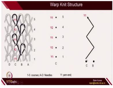
Before I move on I just want to recollect the yarn path which is being followed in a warp knit structure. So in a warp knit structures we have seen like for the same needle in every alternating course it is catching different yarns. So for example if you see this needle number C in first course it is catching Y1 yarn in second course it is catching Y2 yarn, third course it is catching Y1 yarn.
