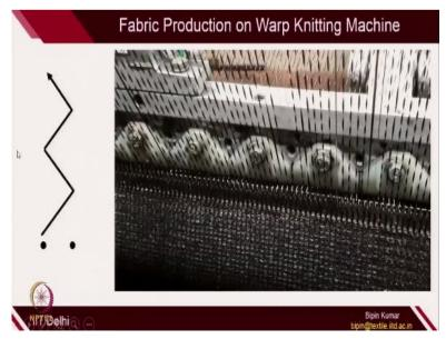
So this is the fabric production in a slow motion I hope you can you can see it moves from left to right and then right to left. So left to right and then right to left so this is how it is doing. So left to right and right to left okay so it is shifting laterally left side and then right side. So this is how the guides are actually changing the direction of yarn in every subsequent courses.
