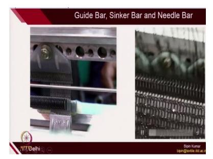
So you can see it here exactly those functions are happening here on the latch needle we are using latch needle here. So the guide is swinging so you can see the guide is swinging then it is providing the yarn it is shifting laterally it is so the guide is swinging you can see it here then it will provide the yarn and then swinging back and the sinker is also moving in the same fashion.
