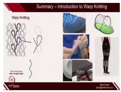
Let's do a quick recap of what we covered in the last lecture. We have seen how loops are connected in warp knitted structures. I already demonstrated you that the yarn in a warp knitted structures follows the length direction that's why it is called warp knitting and each loop is connected with different courses in the structures. So this is how this structure is different from a normal weft knitted structures.
