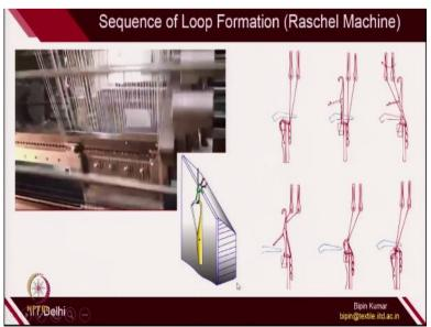
The other technology which is known as raschel machines. The sequence of loop formation remains same the only difference here is here the role of another bed is important. So right now in the tricot machine you have seen there was sinker which was helping in sinker loop formation, but here there is a additional needle bed just like in the case of V bed you have seen you just create the fabric.
