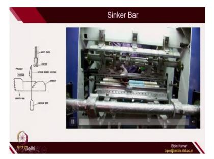
So let's see first fixing of sinker bar. So I am fixing the sinker block which I showed you so this is the sinker block so this is the sinker which I am keeping in my hand and I am fixing on the machine. So you can see it here so this is the sinker I can fix it there is a hole on the entire bar I can put that block in that hole and with the help of screw I can fix it on the machine. So the sinker is now fixed, sinker block is fixed.
