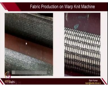
So this is the actual condition where you can see this is happening each guide is carrying the yarn and the fabric is being formed. So you can see this is the yarn and the guides is there they are supplying yarns to the needles in alternating courses. This is the very dense fabric
