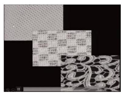
There are different types of fabrics that can be created smaller mesh bigger mesh and this is crochet from so you can see the mesh size is much, much smaller. So these are the types of fabrics that can be created on this type of machines. It again depends on how you are providing yarns and how the guide bars are moving. So the guide bar movement is very, very important in deciding the fabric structure.
