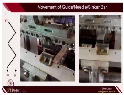
So here you can see how multiple guides, multiple sinkers and needles are operating so you can see it here. So the guide bar is swinging so you can imagine this will be providing yarn and the needle is raising up and down to catch the yarn and the sinker again similar to the circular knitting I already described what is the role of sinker especially it is very important for making sinker loop, holding the fabric when the needle is rising.
