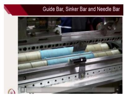
So this is the 3 elements which is placed on the machines so guide bar, sinker bar, and needle bars. So this is one block of needles so this is the needle, this is the needle which is moving up and down. The other block is this is the guide and the third block is the sinker so which is you can see this is the sinker. So 3 blocks you can see it here so one is sinker this first one is needle sinker and this one is guide which is there on the top.
