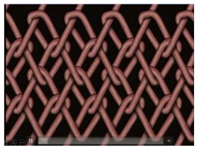
This is the structure which I already described. So if you follow the path of one yarn you can actually see how the yarn path is moving. So this is how it is moving so they are connected with different courses.
