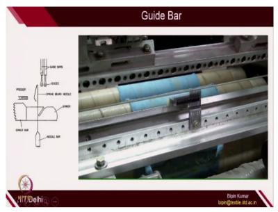
Now the next part is the guide bar so the guide bar this is the guide bar. So here there are 2 guide bars are formed, but I am fixing just one guide bar. So the guide block so I am fixing it so here you there is a holes you can see it here. So I am going to fix in one of the holes the guide. So this is the guide so in reality although you are looking one sinker one needle and one guide.
