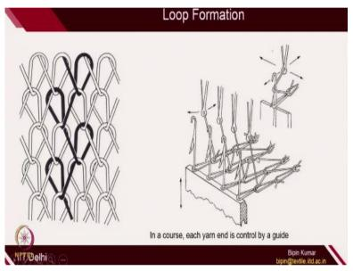
And for providing yarn to each needle we have individual guides and these guides actually keep changing the location in every alternating courses. This is how you define a design a very simple warp knit structures. So the bottom line is the role of guide is extremely important because the movement of guide in subsequent courses will decide you how the loops in the structure will look like and what type of fabric designs you actually want to create.
