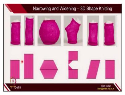
Another thing which is very popular in knitting is 3D shape knitting. So not only V neck and round neck we create but also we can use the concept of narrowing and widening to create 3D shape knitting. So for example if you want to make a fabric pattern which can fits on different architecture different 3D shape object, you can first creates its pattern. So for example if you want to make a circular fabric you just need to create a rectangle because a rectangle can be folded to make a circle.
