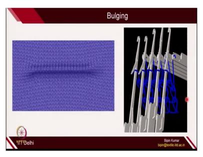
So how do we actually create this kind of bulging a kind of 3-dimensional effect on the fabric surface. So here a simple animation is given to you. So first you create on the both side loops then you keep making loops on 1 of the bed and other loops on the other surface is resting on the back bed. Because of that bigger held loop is being getting created and then you transfer those held loop on the front side.
