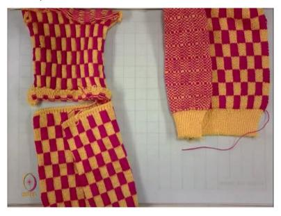
So this was float jacquard. So on 1 side yarns are visible in the loop form other side in the float form. Here on 1 side yawns are visible on the loop form, other side its having the combination of float as well as back loops. So this is because of which it looks like a bird eye. So and this is the tubular jacquard. So I am putting all types of jacquard in 1 place. So that you get better understanding and differentiation of all 3 types of jacquard.
