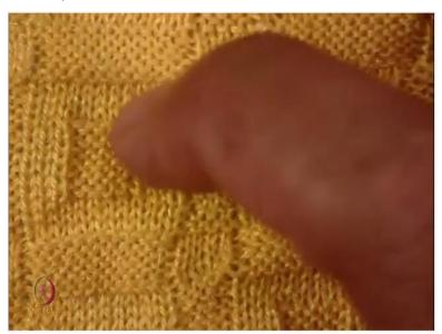
I have another sample of narrowing and widening with link design. So you can see so the fabric just now I told you a bulging effect. This is not the bulging effect but you can see some kind of 3D projection on the loop surface. So this is this is developed by link design. So you can see if
