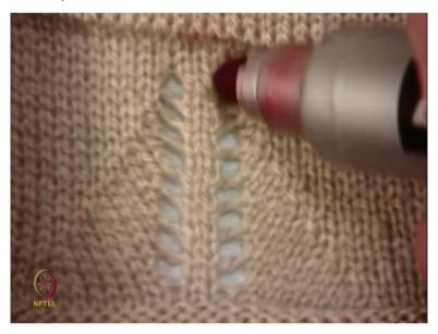
So in pointelle, I am going to show you the pointelle on the fabric structure. So if you see this fabric pattern the different patterns are there I am not going to explain all of these. We will go step by step, let's first focus on this holes okay. So these holes has been created. So we need to observe what exactly the needles are doing on the machine. So these holes are actually pointelle design. So if you if you try to enlarge, so this is how the holes will look like okay.
