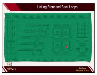
The other complicated designs are also possible. For example, here linking front and back loops you can see you can get any architectures aesthetically it looks very good. So if you want to give some pattern on the fabric surface you can play with the front and back loops. So I have 1 small fabric sample also with me. I can show you how linking front and back loops can give you a different appearance on the fabrics.
