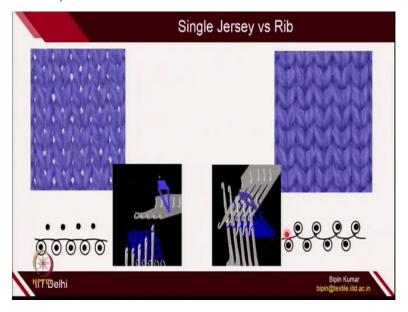
So on the machines, we can create rib design very simply. This can be created on a manual V bed machine also. So if you see single jersey fabrics where the loops are created on 1 bed and double jersey fabrics where the loops are created on both the bed. So if you see the fabric appearance here you can see there are holes because its a single jersey fabrics not that dense. But if you see the double jersey fabrics it is very denses because you have multiple loops on the front and back side.
