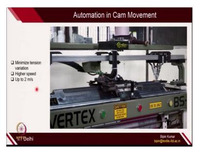
And because of that you have minimum tension variation. And the carriage speed can also be controlled and we can reach up to 2 meter per second. So many thing can be solved because of simple advancement. First of all, this movement will always be uniform. So the tension variations will be minimized the second because it is motor controlled, so you can increase the speed of the motor depending on the requirement. And you can go from slow speed to higher speed.
