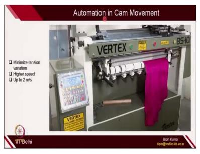
So the first advancement was automation in cam movement. So every manufacture wants limited interference with the operators. Because when there is operator operating the machines, there could be tension variations because of the carriage movement by the hand. First advancement in the machine was done in the automation of the cam movement or the carriage movement. So here you can see the carriage is moving with the help of electronic motors.
