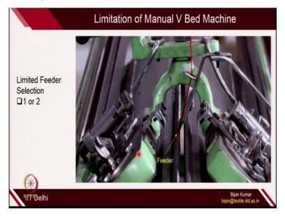
So you have seen the feeder is actually carried by the cam jacket where the feeder is coming and this is the feeder point. And this supplies the yarn in the noodles on the bed. And in normal machine manually operated you have maximum 1 or 2 feeders. So you can play with 2 or 3 colours at max. And we cannot have more than 2 or 3 feeders on the machine. This is again a problem.
