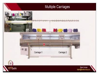
The other innovation from the productivity point of view is the number of carriages. So on 1 of the machine I just showed you the videos. So here 1 carriage is moving okay. Some portion of the bed is not working at all. So if you want to increase the productivity, you can play with multiple carriage on the same bed. So 1 carriage will be making 1 set of the fabrics, other carriage will be making other set of the fabric.
