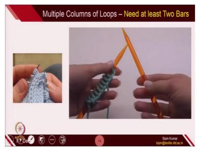
You actually take the 2 bar and one bar actually supports the old loop and the other bar creates the new loop and take the old loop. So, the first bar actually holds the loop and the second bar actually creates the new loop and we keep transferring the old loop from one bar to other bar. Let's see this video, which, through which you would be able to (Video Starts: 18:25) understand carefully.
