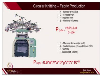
So, in the last lecture, you have seen the production on circular knitting machines. We derived 2 formulas, production in meter per hour and production in kg per hour. So, you do
