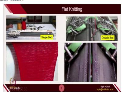
So here, 2 machines we have already seen in previous weeks, single bed machine and double bed machine. (Video Starts: 01:33) So, this is the double bed machines where there are 2 carriers for 2 beds. And they are just moving from one side to other side. (Video Ends:
