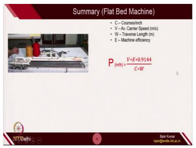
The derivations, you can find it here. Production on a flat bed machines is equals to velocity of the carrier; E is the efficiency; C is the courses per inch; and W is the traverse length. It means, how much the carrier traverse on this bed. So, this is the formula. Let's derive this formulas. It is a very simple steps. And then, you will able to figure it out, how this formula has come. So, let's see the derivation.
