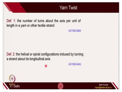
So, twist; if you see the definition of twist as per standards, it is the number of terms about the axis per unit length of the yarn or other textile strands. So, if you take a bunch of fibers and if you try to start turning those fibers along the yarn axis, that is called twist. It is expressed number of turns per unit length. So, the other thing is the helical or spirical configuration induced by turning a strand about its longitudinal axis.
