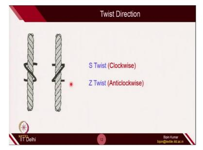
So, in twist, there are 2 terms which is quite commonly used. So, you should also be careful about the kind of twist which is imparted to the yarn, whether it is S-twisted. So, if you see here, here the nature of spirality is along the S direction. So, this looks like S. So, if the yarn is twisted in clockwise fashion, this is S-twisted. And if the yarn is twisted in anti-clockwise fashion;
