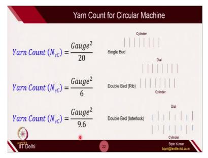
So, here for circular machine, here are some of the useful relationship. So, for single bed, when you have only cylinder, no dial, then the **yarn count** = **gauge**<sup>2</sup>/20. In double bed, when the needles are in rib setting or rib gating, when you had cylinder and dial, then, the **yarn count** = **gauge**<sup>2</sup>/6. Please remember, these yarn count is representing in English count.
