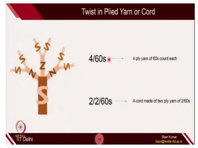
So, in twist in plied yarn; so, the twist which has to be imparted, it must be, the direction must be the opposite of initial twist. So, whenever you have, let's suppose, here you have S-twisted plied yarn. Then, when you are combining these is equals to twisted plied yarn, we need to apply Z-twist. And when you are combining Z-twisted plied yarn, then we have to impart S-twist direction. So, this is again some common things which is found in textile yarns.
