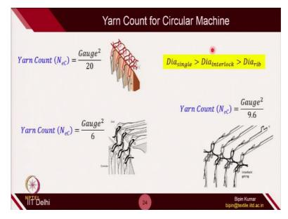
So, if you see single bed, there are lot of space available on the front side of the needle. So, that's why you can play with thicker yarn diameter. But if you see the rib; because of the placement of dial bed and the cylinder bed; so, there is limited space available in double bed machine. So, in, that's why, if you see rib machine and interlock machines, the yarn diameter will be always lesser than the yarn diameter that can be used on single bed machines.
