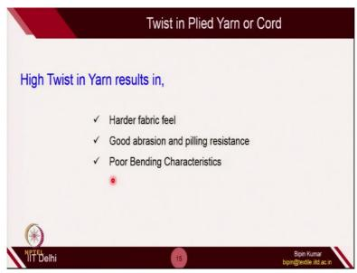
High twist, if you use, you will feel the fabric is little bit harder. It will result in good abrasion and pilling resistance, but unfortunately, it has poor bending characteristics. So, you will realize, when you are dealing with very high twisted yarn in knitting. And in knitting, bending of the yarn is the first criteria. Because, the, if you see the needle movement, it is actually catching the yarn and bending it.
