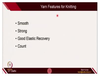
Especially, if the yarn is very, very rough, then you can have the problem of abrasion with the yarn needles or the trick, the trick on the bed. And there, because of that, the fly can generate. So, smoother yarn is better, because it will keep watch in the fabric formation and less fly will generate. And also, the friction will be less. So, there is less rubbing of the machine parts. Yarn should be sufficiently strong.
