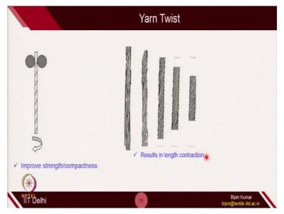
So, in reality, twist is used to improve the strength and compactness. But, too much twist or turning of the fibers should also be avoided. So, for the knitting point of view, twist is extremely important. Because, if you use highly twisted yarn, there might be possibility that it may not bend properly and the loop geometry will be distorted. So, twist as well as count is extremely critical and it should be in certain range, so that it can run smoothly on the machine.
