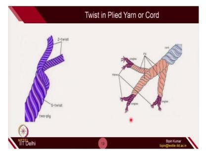
Twist of plied yarn or cord yarn. So, you have seen the plied yarn where 2 or more yarns are twisted together. Sometimes, it might be possible that you can twist 2 plied yarn. So, you can see here, this yarn itself is a plied yarn. And when you are twisting plied yarn to make cord; this is called twist in plied yarn.
