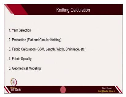
So, let's start calculation part. So, in this particular category, I have divided the knitting calculation into 5 segments. So, first we will talk about the yarn selections. Yarn selections means, you have seen the machine gauge varies, machine technologies varies; so, we cannot run the same type of yarn in all the machine gauge or all the machine technology. So, definitely we need to choose the right yarn or right yarn count for a particular machine technologies and gauge.
