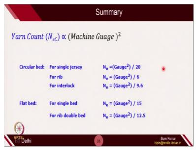
So, this is overall summary of, that yarn count is related with machine gauge square, but depends on the technologies that you are using. For single jersey, **yarn count = gauge<sup>2</sup>/20**. In circular bed, for single jersey flat bed **yarn count = gauge<sup>2</sup>/15**. If you see rib interlock and the constants are keep getting different. And this comes with experience. Let's do a simple
