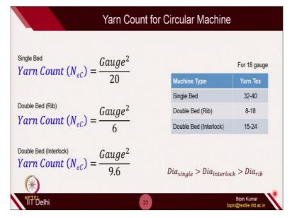
So, if you use this formula, and based on the knitting experience, this is some of the yarn count in tex, which is found suitable for single bed, double bed and double bed interlock and rib machines for 18 gauge. So, if you have 18 gauge, you can see single bed, you can use 32 to 40. So, the range is there, it is not hard and fast rule that you need to have exact same count. You can play  $\pm 4$  depending on the machine technologies.
