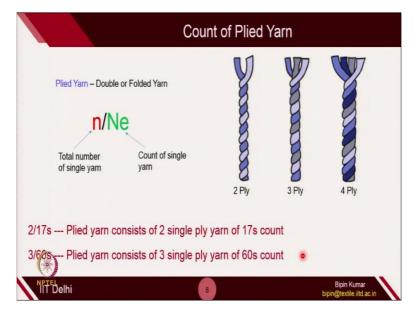
We have also count of plied yarn, which is quite useful, especially if you see sewing yarn and even in knitting yarn also; sometimes we use 2 ply, 3 ply or 4 ply system. Plied yarn is actually double or folded yarn. So, when you take 2 yarns and if you twist together, then you can generate 2 ply, 3 ply and 4 ply, depending on how many yarns you are twisting. Plied yarn actually denoted by this way.
