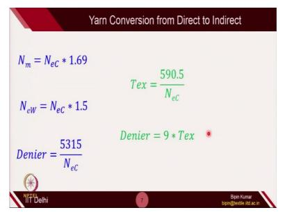
Or you can follow some of these formulas to directly convert from direct to indirect. So, for example, here metric count is connected with English count. So, NeC is the **English count \* 1.69.** So, if your yarn count is given in metric form, then you can simply multiply 1.69. Worsted count, English worsted count is connected with English cotton count is into 1.5. New=Nec\*1.5 So, English count and worsted count is connected by this relation.
