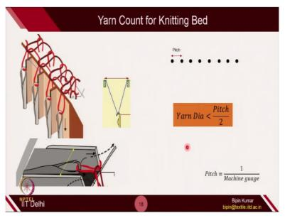
So, if you see the yarn count for a knitting bed. So, in a knitting bed, we have seen the tricks are there and the needle moves inside the trick by catching the yarn. So, you can see here, the needles is moving this wall inside the trick. So, trick is created by the trick walls. So, between two trick walls, the needles is moving. So, these are the trick walls. So, you can see this wedge. So, these represent the trick walls.
