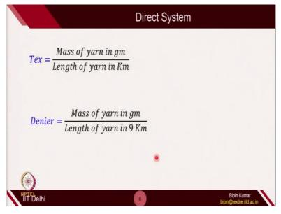
In direct system, this is more direct. So, you will just take the common length of the yarn and you measure the mass. So, tex is described as mass of yarn in gram and length of yarn in kilometer. So, you take 1 kilometer of the yarn and you measure its weight; that is the tex value. In case of denier, you take the mass of yarn in gram, length of yarn in 9 kilometers. So, these are the direct system.
