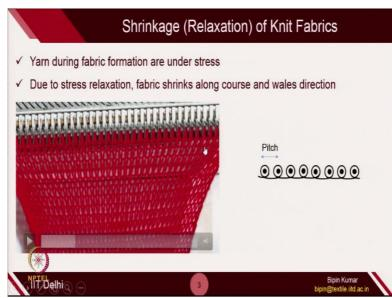
(Video Starts: 03:09) So, if you see the fabric on the machine, you apply dead weight at the bottom. And you keep running the carrier from left to right and right to left. So, yarn during the knitting are extremely in stress conditions, because you are pulling the fabric from the bottom. So naturally, the fabric is under stress condition. Each yarn, you can see, each yarn are being pulled at the bottom side.
