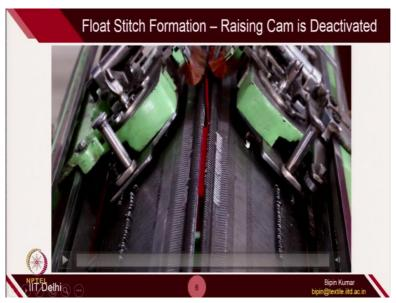
So, this is how I do. So, you have 4 float stitches, 2 for each bed. So, these 2 are operational, when you are moving the carrier from one side to other side. When you are reversing the direction of carrier, the opposite 2 cams raising cams will operate. So, at this moment, in this video, (**Video Starts: 03:54**) I am pushing inside. So, in that case, I am making sure the raising cam has suppressed inside.
