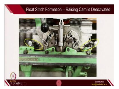
So, for float stitch, raising cam has to be deactivated. So, this is the location. You can push this metallic bar inside to make float stitches.
