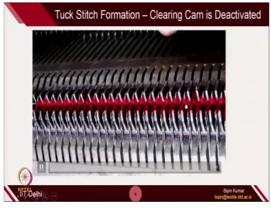
So, this is how it works. So, (Video Starts: 02:40) the moment you press it from one side to other side, you basically suppress the clearing cam. And then, you can run the machine for. This is only for one direction on one bed. So, similarly, you have 4 clearing cam setting. 2 for each bed. For left to right direction and right to left direction. And similarly, for the other carrier, on opposite bed you have 2 cam settings.
