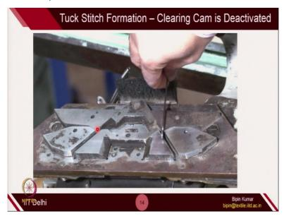
Let's see, actually this is a small video (Video Starts: 24:44) how you can; so, this clearing cam is in a deactivated position. So, it actually raised and then goes like this. So, you can see here, raising cam is allowing it to rise, but clearing cam is not activated, so it will just go straight. So, in a machine, for 2 traverse, there are 2 clearing cams from one side. So, this is, now this time we are (Video Ends: 25:09) forcing this clearing cam to go down.
