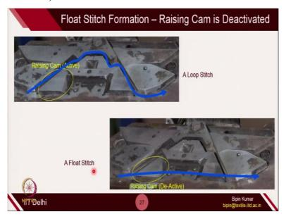
Now, let's see, on the cam jacket what need to be changed to create this particular held loop? To create float stitch, the raising cam on the cam jacket has to be changed or you have to play with the raising cam. So, if you see this particular raising cam, this is in active position. So, when the needle butt is coming from the left side, it will hit the raising cam and it will go up and follow the cam profile.
