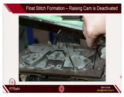
So, I have a the video where you can see what is exactly happening. So, I have pressed this raising cam inside, so that it will not hit the needle butt. (**Video Starts: 42:09**) So, you can see this is in downward position. So now, the needle butt, nothing is there. So, it will not rise, it will just pass. So, if it is not rising, naturally it will neither catch the yarn, neither it will clear the old loop. (**Video Ends: 42:25**)
