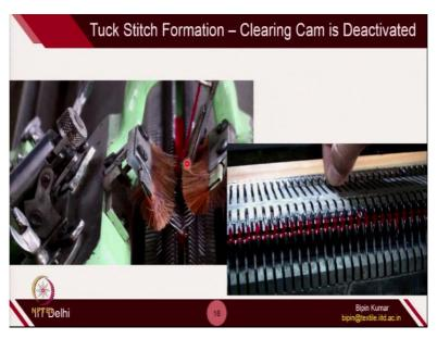
When I am pushing this with my finger; (Video Starts: 26:39) so, this is how you push it. So, when you do this, the clearing cam on the back side of this cam jacket goes inside. It will not allow the needles on this particular bed to rise and clear the old loop. Okay. There are actually 4 position where you can play with the (Video Ends: 27:04) clearing cam. So, on each bed, the jacket is moving from left to right and right to left.
