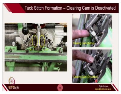
The cam jacket will actually look like this. So, if you see this cam jacket, there are 2 knobs, metallic knobs. And for one when the cam jacket is moving from right to left and the other when the cam jacket is moving from left to right. So, this is there to either raised or depressed the clearing cam on the back side of this cam jacket. This is the active position of the metallic bar with in, on which the clearing cam is at active position.
