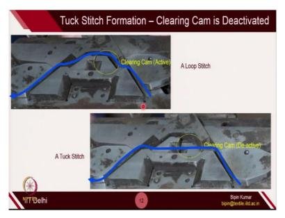
To create tuck loop, we have to deactivate the clearing cam. So, I hope, if you remember this photo; this is the cam profile of V-bed machine. So, this is particularly the clearing cam; if you remember. So, this is the raising cam; then clearing cam; then stitch cam; and this one is the guard cam for V-bed machine. So, in one of the position, you can see, the clearing cam is actually raised on the surface.
