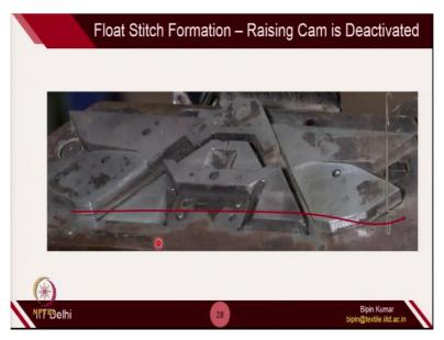
Let's see how things are moving here. (Video Starts: 41:45) So, if you see the needle, needle just follow this particular path. (Video Ends: 41:49) So, needle is not rising. So, needle is just remain in idle position. So, this is how the float stitch is created.
