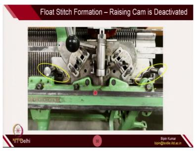
This is the cams where how you control the actually floating cams. So, these 2 bars, when you push inside, actually you are deactivating the needle cam. So, when the cam jacket is moving from left to right, and then you, if you push this inside, then you are creating floating loops. And when you are moving from right to left, then this cam has to activate for creating float stitch.
