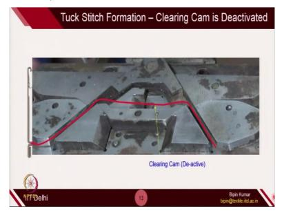
So, this is the clearing cam which is in deactivated positions. So, in deactivated position, you can see, it is being pushed inside the plane. So, there is no projected metallic surface which can hit the butt of the needle. So, when the cam traverse on the machine, the butt will follow this particular path. It will not go above this clearing cam, because clearing cam is deactivated. (Video Starts: 24:19) This is the actual path.
