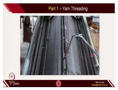
So, the first thing. In front of the machines, you have to supply yarn. So, the first part, we are going to see how yarn is being thread in this particular machine. (Video Starts: 01:35) So, let's see how the yarn is being thread. So, this is the yarn. Similar to the single bed machines, here in V-bed machine also, the yarn has to pass through guide and tensioner system. So, it has first passed to the first guide.
