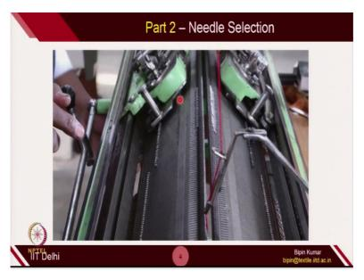
For the selections, let's see. So here, (**Video Starts: 03:25**) how you can select the number of needles on each of these beds. So, this is the front bed. So, you can simply push the jack from the back side and it will push all the needles on the top side. So, in this way, the position of the butt; so, each of these projected part is actually one of the needle butt. So, in this way, you can place all the needle butt in one that particular location.
