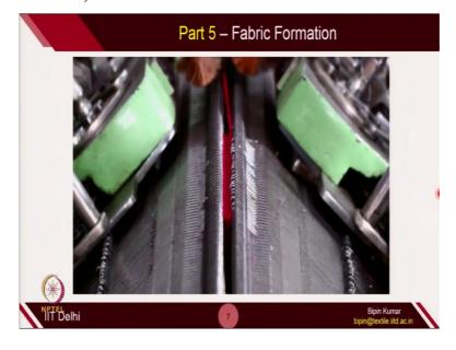
So, this is the (**Video Starts: 07:44**) process you can keep taking the cam jacket from left to right, right to left, depending on how many courses you want to create. So, each traverse will create 1 course. This is how we make the fabric in a V-bed machines. And V-bed machine, as I told, this is one of the most popular machines, because this gives you lot of flexibility. You can any time close one bed and operate on a single bed machine.
