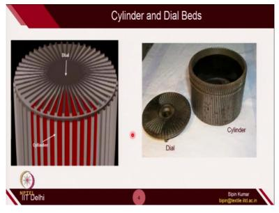
Here you can see, here the dial, the slots or the tricks is created in radial directions. So, you can see here, this is the radial direction. And the slots are created. In each of these slots, you fit needles along the radius. So, the direction of movement is along the radius. And the vertical cylinder, again the slots are created. And on each of these slots, you fit needles. So, this is how the arrangement of 2 beds are done in circular knitting technologies, which is having 2 beds.
