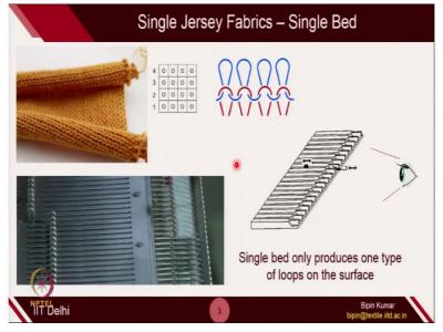
To understand this, if you will see the nature of a single flat bed, it can only produce technical back or front loops on the surface. So, this surface which you are looking at, it is only consist of head and sinker part. So, naturally, this symbol indicates technical back side. So, in technical back sides, all loops which is denoted here in blue segments are going behind the red loops. So, it is being formed on the back side of the loop.
