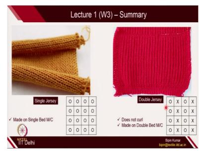
One was single jersey fabric, which I just introduced to you, which is usually made on single bed machines. In a single jersey fabrics, you can either see technical back loop on one side of the surface; and if you flip that surface, you will see technical front side. And you can see how difficult it is to work with single jersey fabrics. So, the moment you relax this fabric, it will try to curl from the edges.
