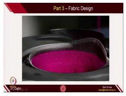
So, once the needle start catching, you can any time replace any color of yarn and you can create different stripes. So, this is useful in design purpose. So, you might have seen the socks of different stripes. Also, there are lot of complicated designs are there. Such machines are also useful. But in this machine also you can any time change the color of the yarn and you can create different designs.
