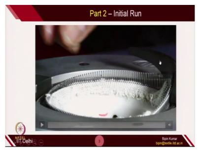
Let's see initial run. Initial run is little bit difficult because, to catch the yarn, the latch of the needle need to be open. We have, there was no old loop, so it was difficult to predict, like all the latch of the needle will be open across this circumference. So, we need some kind of brush to open the latch for all the needle so that it can keep catching the yarn in during the rotation. So, let's see. (Video Starts: 04:54)
