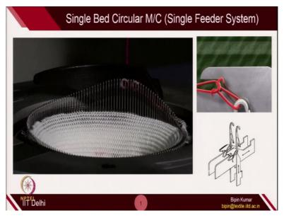
Just a quick recap. I hope you remember this video. (**Video Starts: 00:49**) So, how this particular single bed circular machine is utilizing the yarn and creating fabric with the help of knitting action. In this particular machine, we also have seen how the sinker also helps in loop formation in holding, releasing and making loop. Okay. So now, we are going to see how we place yarn in this particular machine; what happens at the initial stage;
