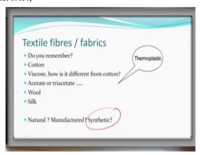
These are thermoplastic fibres, because the reason why cotton cellulose is non thermoplastic, that reason which is the intermolecular hydrogen bonding, that reason has been basically removed by substituting acetate groups. So, then you have wool, interesting natural fibre. Silk, another
