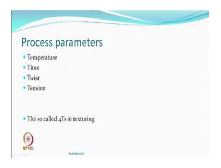
So, we look at the process parameters there are 4 Ts of texturing; the temperature, time, twist and tension. So, you have a possibility of changing any one of these on the machine and therefore, optimise the process. So, temperature, tim, e twist and tension the 4 Ts of texturing.
