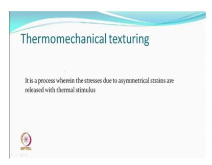
So, what is thermo mechanical texturing? It is a process this sentence you may just try to remember, it is a process wherein stresses due to asymmetrical strains are released with some thermal stimulus. Asymmetrical strains; obviously, different portion of the filament
