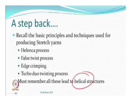
And so if you recall we had talked about stretch yarn which can be produced by Helenca process; which is a batch process. But it gives you helical structure because we are using twist, then there is a false twist process the twist is still being imparted, but in a manner which is slightly different this also gives you the helical structure.
