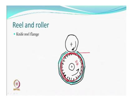
So, what you do is a knife reel flange. So, you have a drum type of thing with a blades like knifes are protruding out all over right. So, you can rotate this. So, these are knife; sharp knife on a flange arranged in this manner. So, there is the blade like going this you turn this, there is another blade, there is another blade, and there is a gap.
