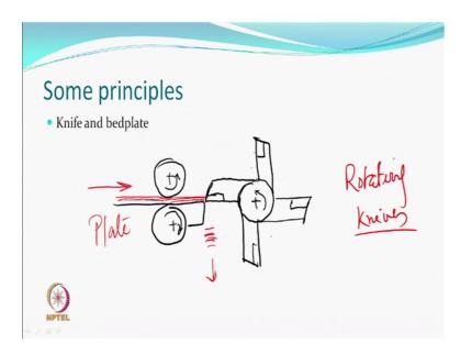
So, you have to cut them some of the principles of cutting call a knife and a bedplate. So, you have a bedplate here this is a plate over which there is a fibre tow is there may be spread over a plate it is being fed and then this is a system of four knife let us say very closely the come and cut for example, and the fibre will keep following.
