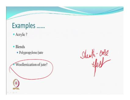
So, what kind of an example possible; so, there is a yarn which is available in the market which we call as the based on acrylic fibres, but you can have blends, polypropylene jute. Now you how does polypropylene and jute would work? Are we saying polypropylene will shrink and jute will not? That can also happen, but then polypropylene much shrink more.
