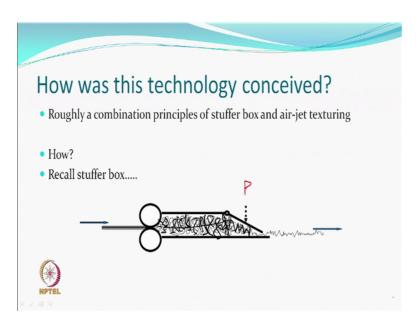
So, this technology that roughly employs principles of stuffer box and air-jet texturing. In some sense stuffer box produces yarns which are in the category of modified stretch yarns, air-jet texturing produces yarns which are bulked yarns.
