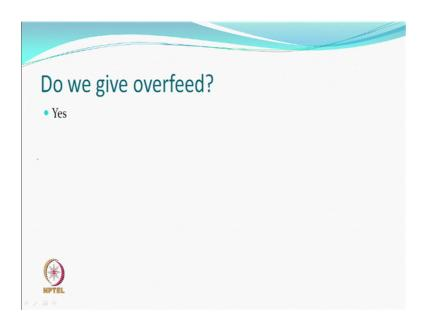
Do we give over feed? Of course, whether it is the air-jet or it is the stuffer box, we are giving or feed. So, over feed will also decide as to what is going to be the number of loop, a number of crimps and frequency of the crimps. Of course, when you say hot
