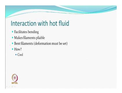
So, common sense also says that after hot air bending, it will become pliable so, becomes easy bending. The bending bent yarn must be made stable so, there has to be a process of cooling the yarn so, that we get the crimps stabilized and so there has to be cooling mechanism.
