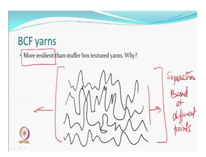
We expect a more resilient yarn, then stuffer box. What it means is that the filaments after separation bend at different points. So, of course, you will have this bulk, you will have stretch. So, these are possible, but because they are not following each other the
