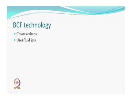
BCF technology wants to create crimps and uses fluid jets and therefore, the fluid jet part learning has come from the air-jet and crimp. That means, you hit the wall and bend that is come from the stuffer box and so this has become more effective and popular. (Refer Slide Time: 06:46)
