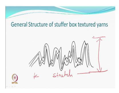
So, we expect that the structure of a stuffer box textured yarn would be crimped not necessarily very uniformly when some the frequency as well as the amplitude may not be uniform. But what happens whenever they bend all the filaments bend together at whatever point they bend so, you get a structure like this. So, it gives you some amount of bulk and some amount of stretch.
