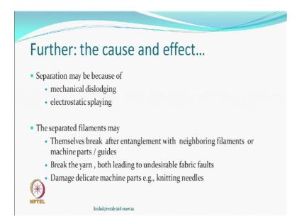
The separation could be because of mechanical dislodging, remember we apply a spin finish and one of the aim of the spin finish is reduction of the friction of course, reduction or elimination of static charge generation and also hopefully keeping the filaments together, some type of a cohesive bonding should be there. But it may not happen because your processing winding, unwinding, passing through guides and it can happen that the filaments can get separated.
