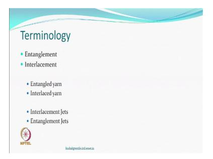
So, sometime the terms could be entanglement or interlacement they mean the same thing, what it means is the filaments have entangled or they have interlaced. The yarn that have been subjected to this process could be entangled yarn or interlaced yarn or the jets which are also used for this process are called interlacement jets or entanglement jets.
