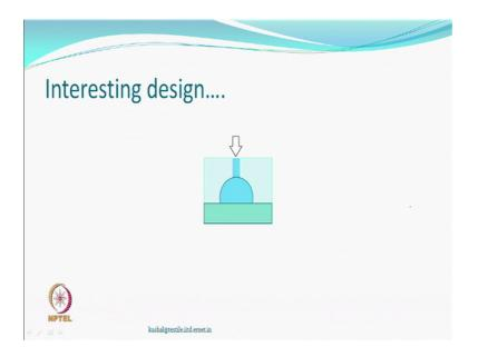
So, the design is like this, semicircular and you see a different color so this is a plate. So, instead of the threading becomes easy, so there is some kind of a plate we just remove it can be moved on one side hinged or pivoted and then you can pass your thread and then closes.
