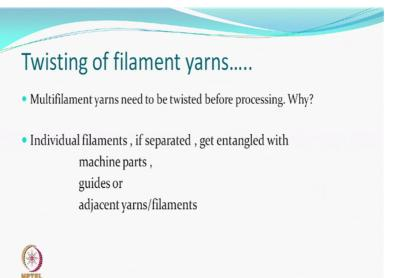
In general twisting of the filaments is done, a parallel bundle of filament in general is not processed because if individual filaments get separated, then they can get entangled with machine parts or guides or adjacent yarn and filaments which obviously, is not a good idea. Therefore, filament yarn industry believes in giving some amount of pre twist very very small just to ensure that the filaments do not get separated and that is a norm.
