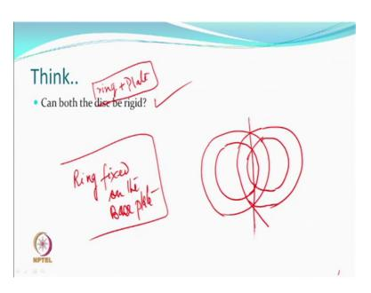
Now, this is interesting. So, one ring, the other ring both are on the base plate, base plate is rigid. Now, we said if there is a rigid body in contact so vibration issues are going to be taken care of. So, both are rigid now, no harm to the fibre, it is not too ceramic surfaces are going to rub the hard surface is away. The one which is going to contact will be a polymers base surface right.
