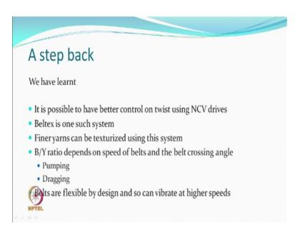
Till now what we have done is that we have understood that it is possible to have a better control on twist using nip controlled vector drives. Beltex is one such system, which was almost similar to hand spinning. And, because of this better control on twist finer yarns can be texturized using this system. Finer yarn means whose individual denier per filament maybe sub denier.
