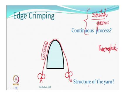
So, another process which is used to produce stretch yarn. Remember we are still talking about stretch yarns; is called edge crimping. And what is edge crimping you take a yarn over a sharp edge, under tension. If you take a yarn over sharp edge under tension and if you want to design something you can let us say it is also easy to understand to begin with, is also thermoplastic yarn. So, you can put a let us say heating device as it moving.
