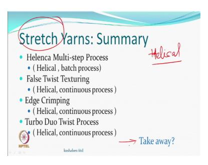
So, let us have a summarize stretch yarns, Helenca multi step process it also gives you a helical structure, but it is a batch process. False twist texturing is a continuous process it also gives helical structure. Edge crimping also gives helical structure as a continuous process and turbo duo we just finished also is helical process, it gives you helical structure. Why? Because the common factor is twit no it is not common factor is that in
