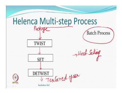
So, what of the process that has been used to produce stretch yarn is called the Helenca multi step process, It is called multi step because there are many steps involved like there is a process which is to be done called twisting. So, it is a multi step process. So, you have to twist so there is one, you remember which other process was also using twist. Last time we talking about the historical perspective you remember any name.
