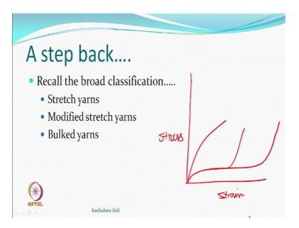
And we remember that the broad classification said that there is stretch yarn and the modified stretch yarn and the bulk yarns. So, you remember what kind of a material will be called a stretch yarn? What type of material will be called a stretch yarn? The one which can stretch up to 300 to 400 percent and the one which are modified stretch yarns would be doing the same thing, but at a lesser stretch ratio.
