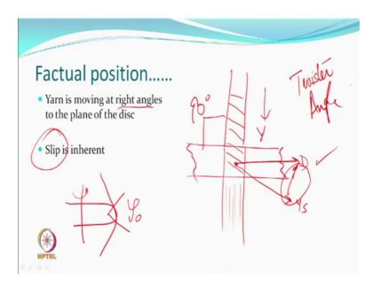
So, current factual position is that you have a disc which is rotating in a plane all right; disc is rotating in a plane. The yarn let us say is coming from vertically from top to bottom let us say. So, this is the disc and this is the disc surface, your yarn is coming vertically but, maybe it is making a wrap angle right so there is a wrap angle.
