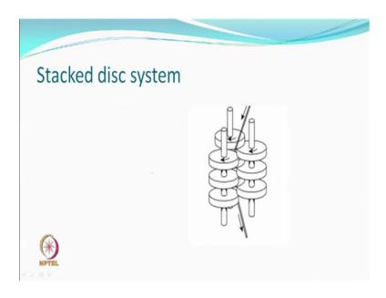
So, 3 axes, 3 shafts or valves and the yarn moves from one side goes on the other is then handle by the second, then the third, then the fourth, then the fifth, then the sixth and seventh whatever. So, this is the problem that I have given you involves only 2 axes system, not 3 axes system and only we are looking at; we are looking at wrap angle.
